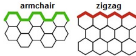
Figure 2.26: Orientation of CNTs. Figure extracted from: Mechanics of Carbon Nanotubes: Fundamentals, Modeling and Safety 46
