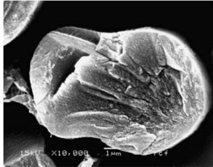
Figure 2.24: Example of SEM image of the surface and cross-section morphology of rayon carbon fiber. Image extracted from: SEM/STM studies on the surface structure of a novel carbon fiber from lyocell 31
