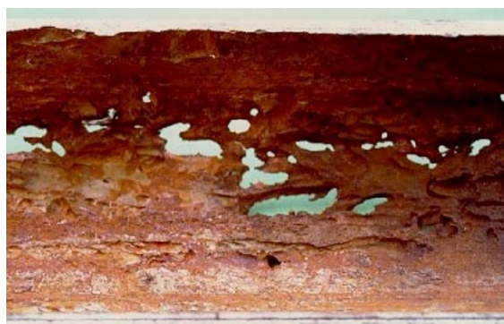
Figure 5. Metal surface attacked by CO 2 corrosion (sweet corrosion) taken 17
