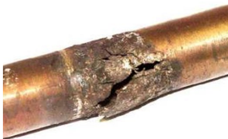
Figure 3. Localized crater-forming corrosion in a good pipeline.
