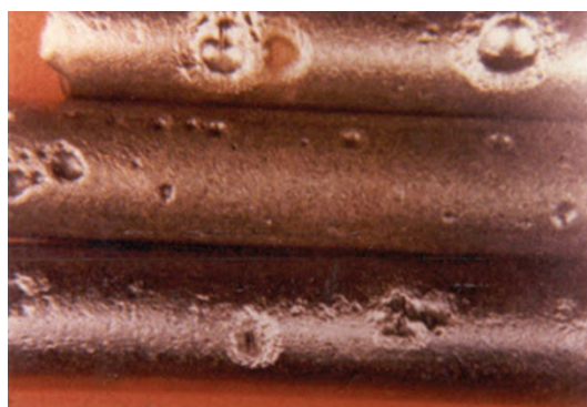
Figure 6. H 2 S-induced corrosion on a metal Surface 17
