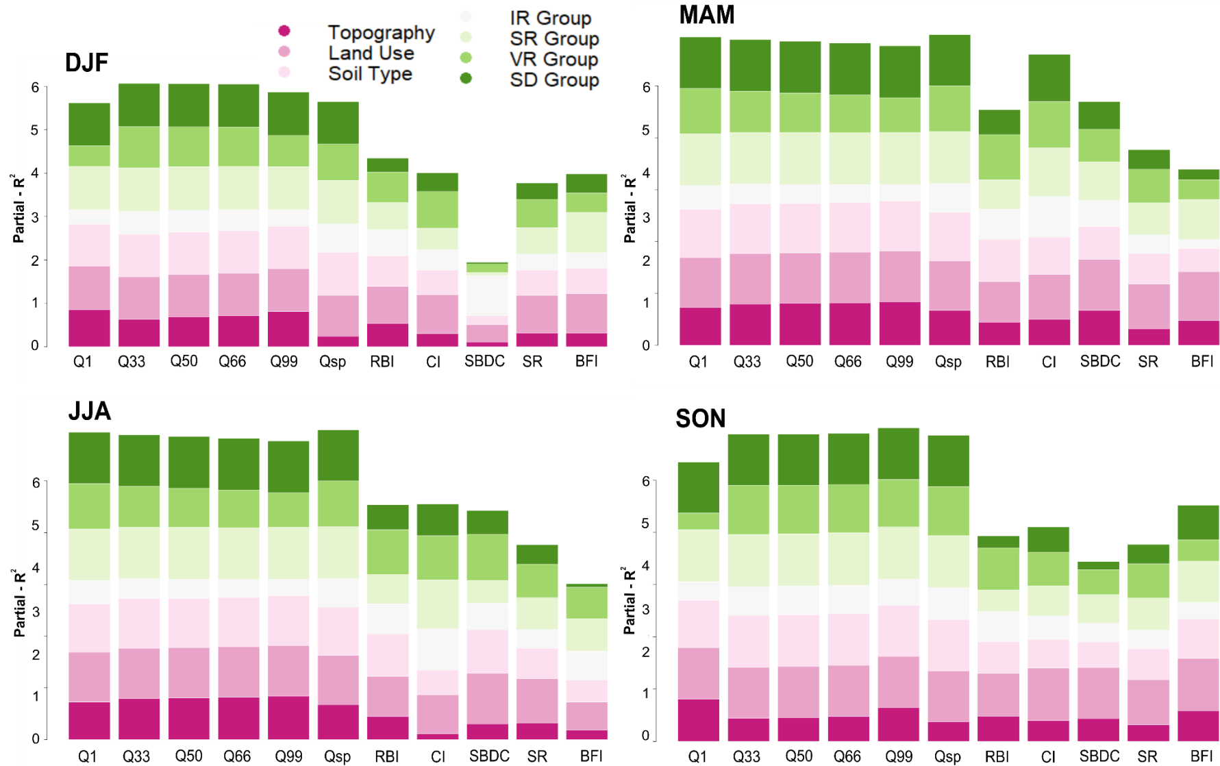
Fig.20. Partial R^2 of different catchment descriptors used in the regression models for Baseflow signatures
