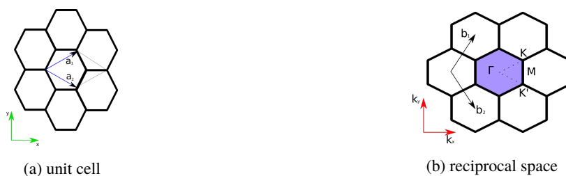
Figure 2.2: a) Honeycomb lattice of graphene with the unit vectors a_1 and a_2 in the real space, and b) reciprocal space of graphene with vectors b_1 and b_2 and the symmetric points \Gamma , K , M , and M' (based on Dresselhaus et al. , 2005)
