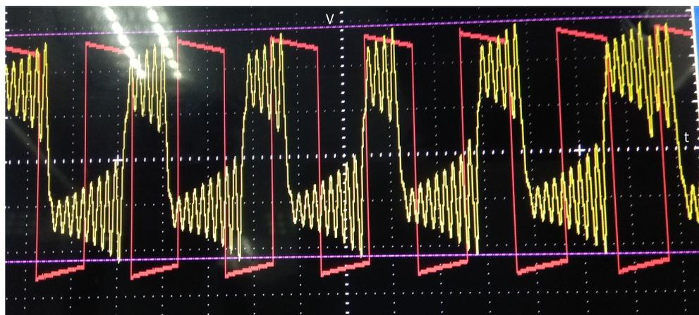
Figure 3.2: Chua signal vs periodic signal displayed in oscilloscope
