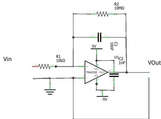
Figure 3.1: Circuit schematic of amplifier circuit<sup>29</sup>.
