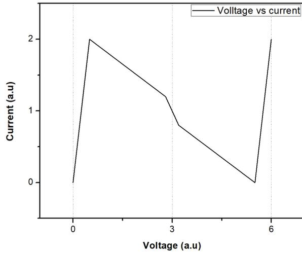
Figure 2.6: Chua's diode Voltage vs Current diagram
