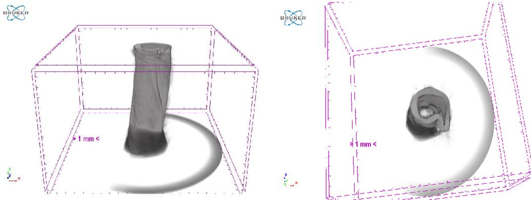
Figure A.2: 3D x-ray image of sample control of dynamic experiment
