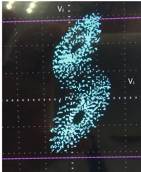
Figure 2.8: Chua's circuit signal measured on an oscilloscope between  $V_1$  vs  $V_2$ .
