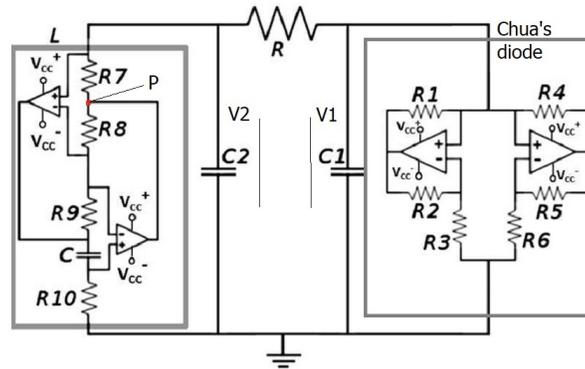
Figure 2.5: Chua circuit basic diagram<sup>28</sup>
