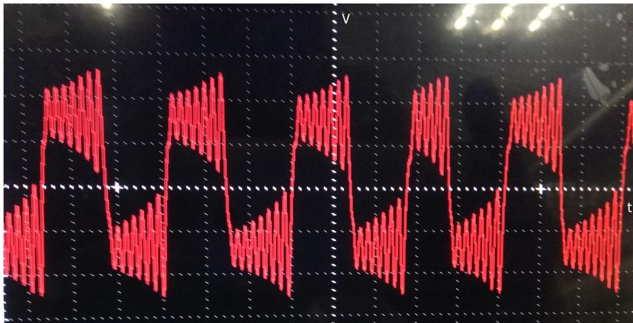
Figure 2.7: Chua's circuit signal measured on an oscilloscope.
