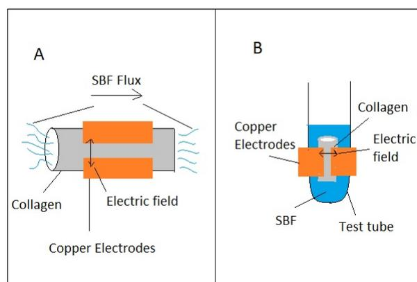
Figure 3.3: Experimental set up schematic, (A) dynamic experiment and (B) static experiment
