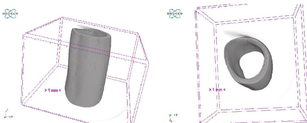
Figure A.6: 3D x-ray image of sample chua2 of static experiment
