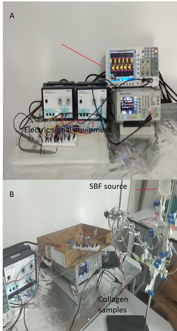
Figure 3.4: Experimental set up, (A) is the experiment ES equipment, (B) is experiment mechanical fluid system.
