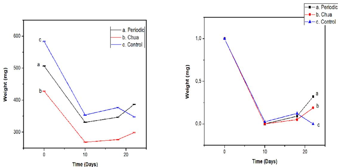
Figure 4.1: Collagen Weight vs Time of treatments: periodic, Chua and control for dynamic experiment, (A) Raw data, (B) Normalized data.
