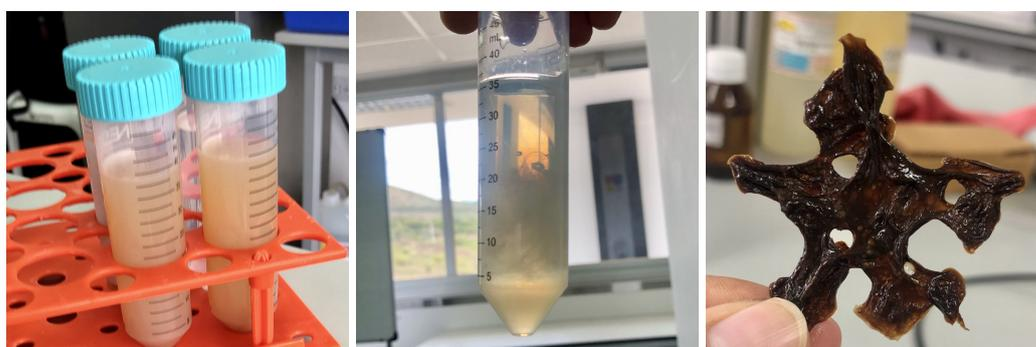
(a) Viscous liquid after filtration. (b) Precipitation with ethanol. (c) Dried pectin.
