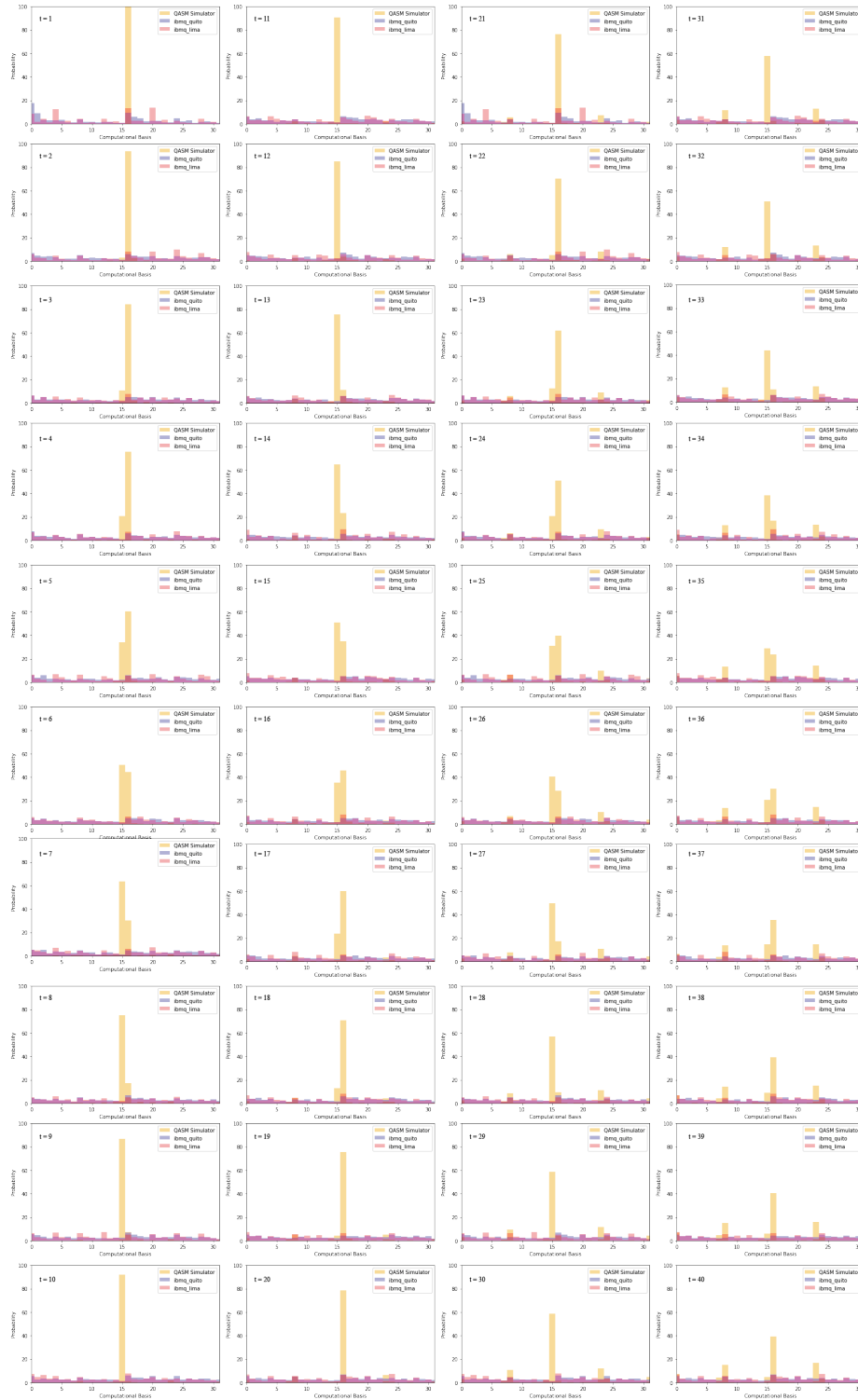
Figure 4.13: Double well potential evolution state's probabilities by using \Delta t = 0.1 [ns], t = 40 [ns], and 1000 shots executed on ibmq-quito and ibmq-lima
