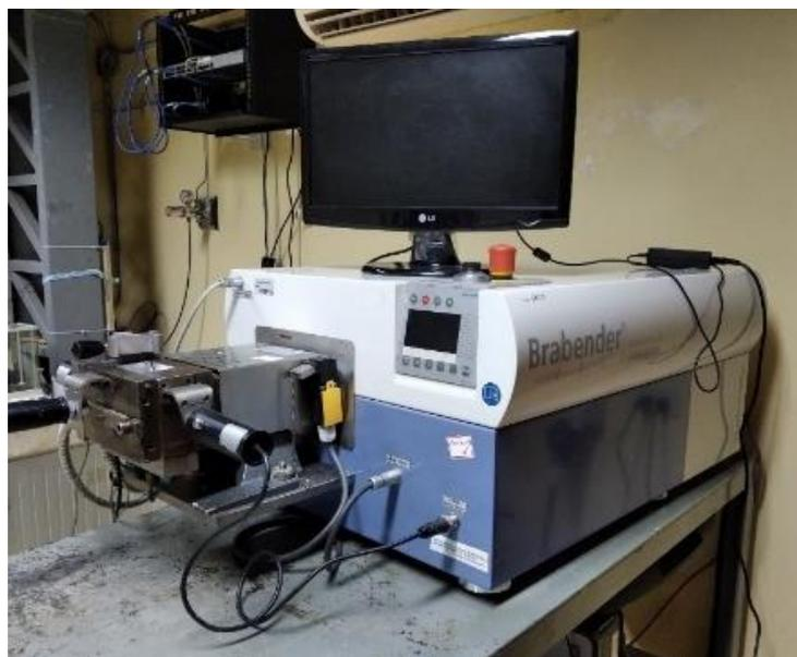
*Figure 8. Brabender Plastograph EC Plus Torque Rheometer*
