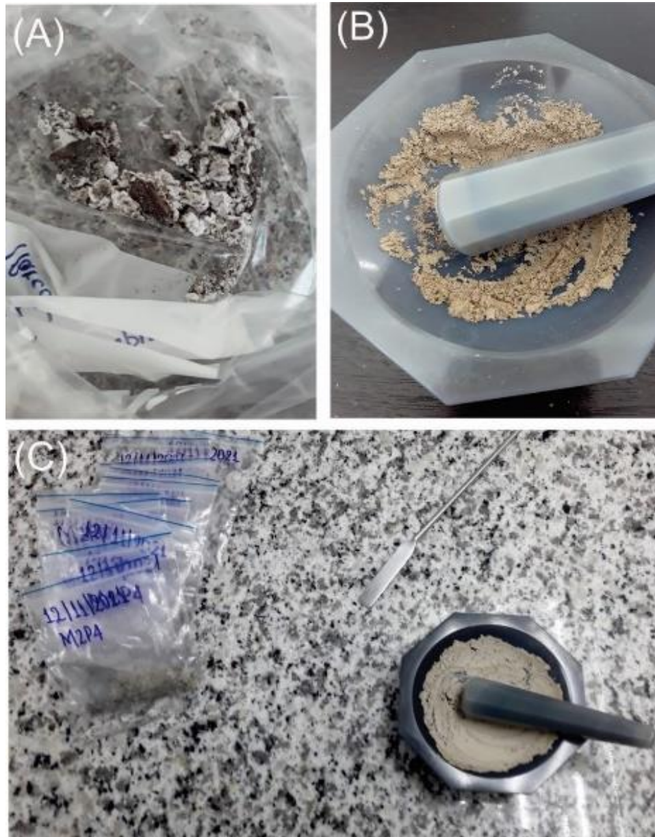
Figure 10. Crushing process (A) Saline samples for X-RAY DIFFRACTION (XRD) analysis (B) Crushing samples in an agate mortar. (C) Samples for X-RAY DIFFRACTION (XRD) analysis.
