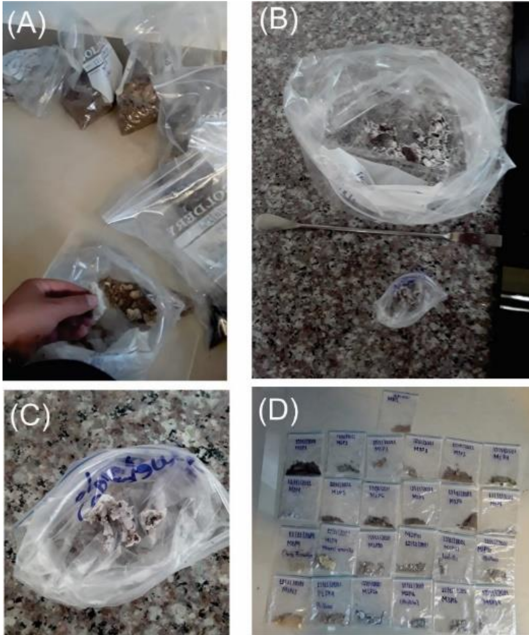
Figure 9. Sample preparation sequence (A) Manual selection of saline structures (B) Separation and scraping of salts. (C) Saline samples collected (D) Samples for X-RAY DIFFRACTION (XRD) analysis.
