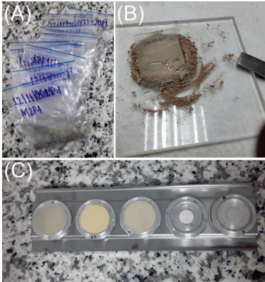
Figure 11. Process before X-RAY DIFFRACTION (XRD) analysis. (A) crushed samples. (B) Preparation in the aluminum sample holder. (C) Samples before X-RAY DIFFRACTION (XRD) analysis
