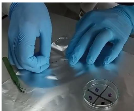
Figure 1.5: Synthesis of graphene by mechanical cleavage of HOPG.
