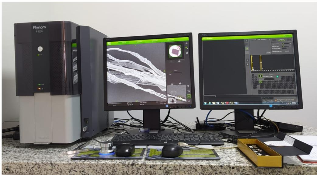
Figure 3.6: Phenom-ProX model scanning electron microscope with software Pro-Suite detector fast SDD at Yachay Tech University, Ecuador
