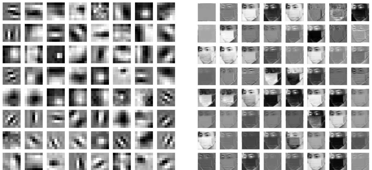
Figure 5.24: All 64 filters of the first convolutional layer with the feature maps they produce.
