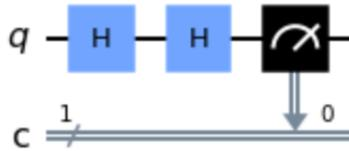
Figure 3.29: Circuit for calibration of the  $\hat{H}$  gate, using the  $|0\rangle$  state.
