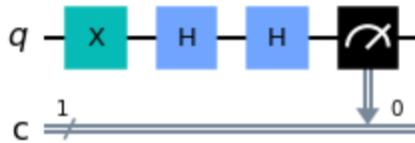
Figure 3.30: Circuit for calibration of the  $\hat{H}$  gate, using the  $|1\rangle$  state.
