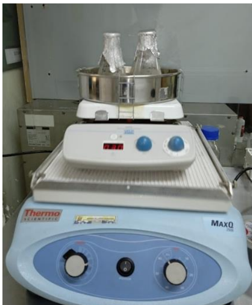
Figure 3. Adapted mechanism to incubate and agitate bacterial culture.
