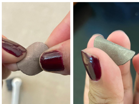
Figure 5.7: Twisted and Bended to a 23 mm diameter electrode.
