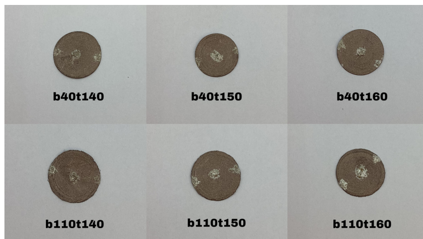
Figure 5.1: Electrodes printed with different temperatures of the bed and nozzle.
