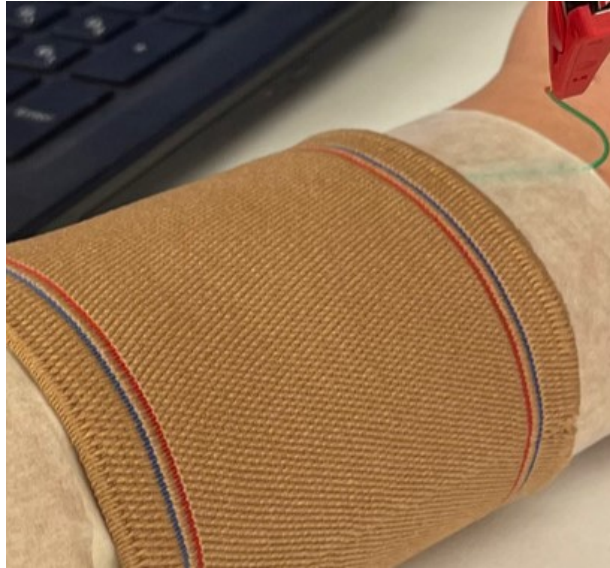
Figure 4.5: Wrist strap to apply force over the dry electrodes
