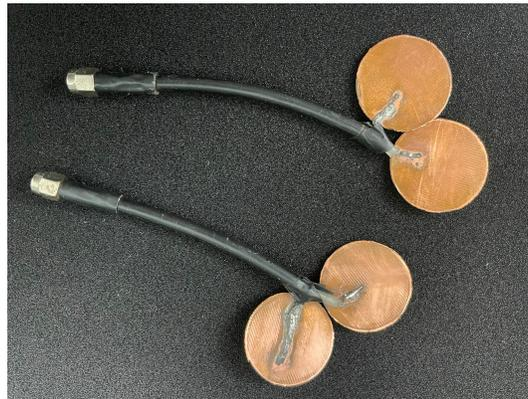
Figure 28: Planar Galvanic electrodes 2.5 cm of diameter.
