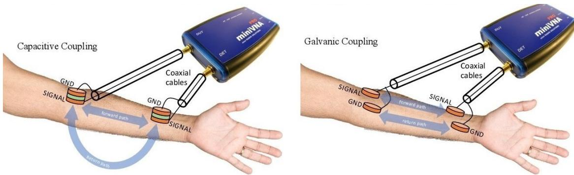
Figure 23: Experimental setup for Capacitive and Galvanic Coupling on a human arm, showing the current paths on human's body.
