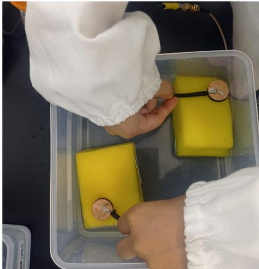
Figure 29: Experimental characterization of planar capacitive electrode at 15 cm
