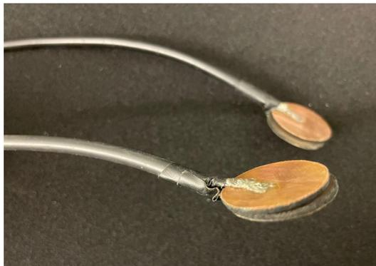
Figure 27: Planar Capacitive electrodes 2.5 cm of diameter.
