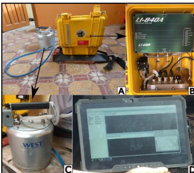
Figure 12. The West System Fluxmeter equipment used for the study. A: The Classic Portable Fluxmeter. B: The AD (analogue – digital) converter and the LICOR® infrared gas analyzer is located inside a box adapted as a backpack to be transported. C: The metallic accumulation chamber (model B). D: The field computer, connected via Bluetooth to the AD converter
