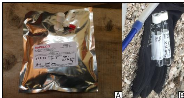
Figure 18. Gas sample collection instruments. A: bag used to take gas samples. B: Vials used to take gas samples.
