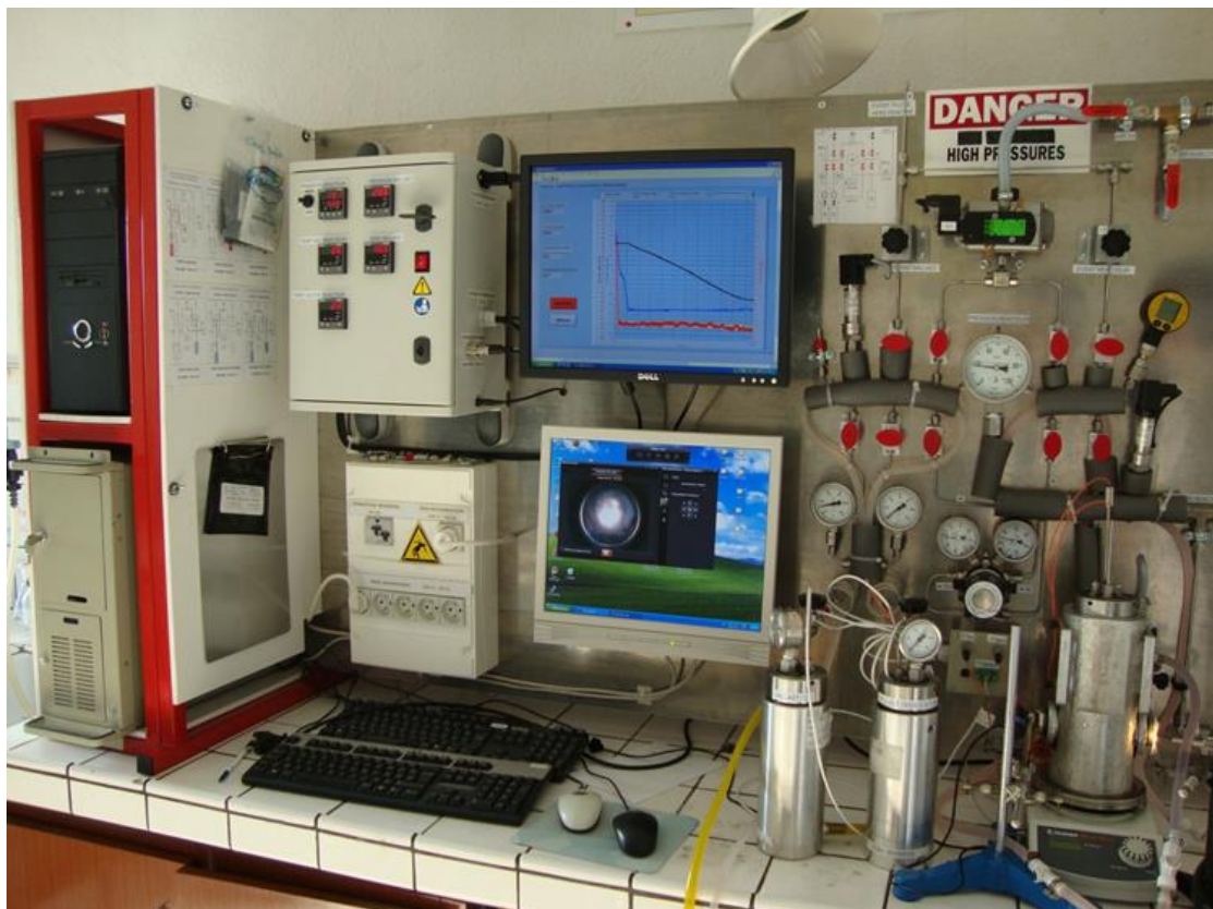
Figure 5. Experimental setup for the analysis and characterization of hydrates (Díaz & Ricaurte, 2021).
