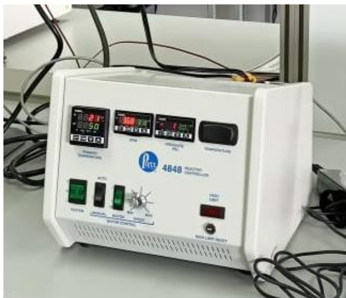
Figure 12. Temperature controller Parr 4848.
