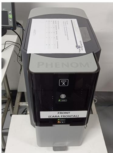
Figure 3.5: Phenom ProX Desktop Scanning Electron Microscope.
