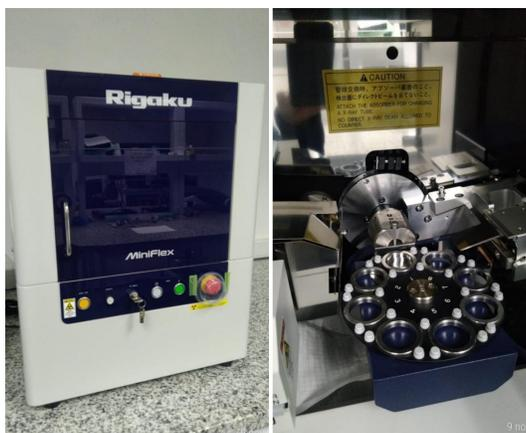
Figure 3.3: An X-ray diffractometer Rigaku, MiniFlex.
