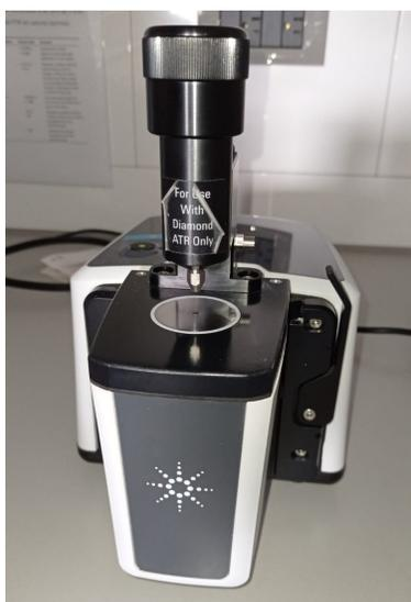
Figure 3.4: Fourier-transform infrared spectrometer Agilent Cary 630 FTIR.
