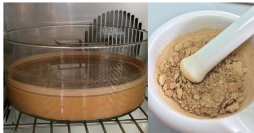
Figure 12: In the left site the drying process and in the right the milling process of the clay.
