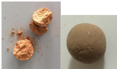
Figure 13: Pellets during mechanical resistance test, at the left a pellet that does not pass the test and in the right a pellet that support the mechanical test.
