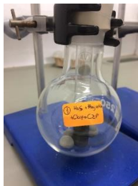
Figure 6: Hermetic system for the test of reactivity, containing the pellets.
