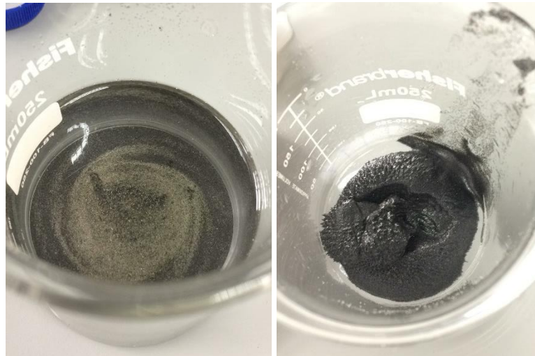
Figure 7: Separation of impurities using a magnet. The right site is before the separation and the left site is after the separation.
