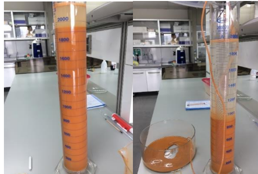
Figure 11: The Bouyoucos method for the treatment of the sample COL-308. In the right side the sedimentation was finished.
