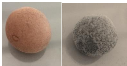
Figure 15: Reactivity test, in the left pellet before the reaction and in the right pellet after the reaction
