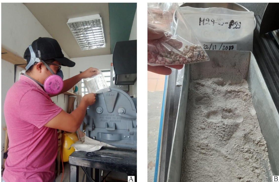
Figure 12. Crushing of samples using the disc mill (A). The pieces must be well dried so the crushing is homogeneous (B) and not mixed with organic matter.
