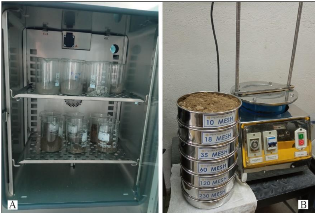
Figure 8. The samples are dried in an incubator at 85° for 4 hours (A). B) After drying, the samples can be sieved on sieves from 10 to 450 mesh.
