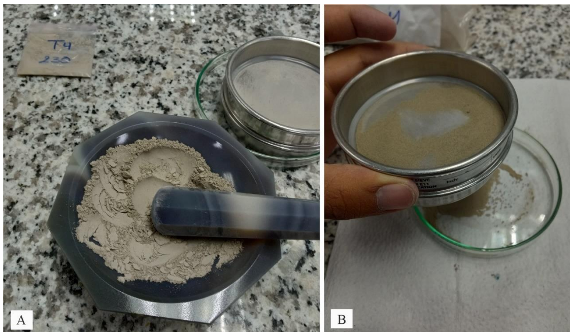
Figure 13. Sample preparation by crushing the agate mortar (A). Samples should be turned into a powder so they are passed on the 450-mesh sieve.
