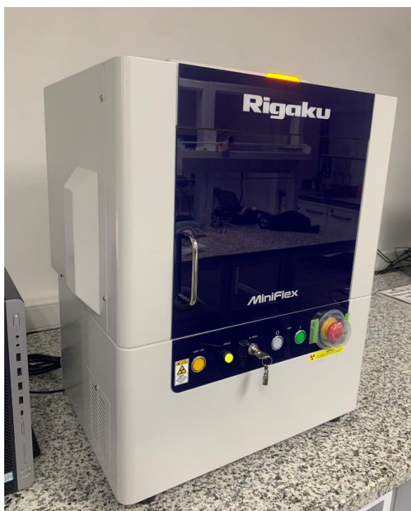
Figure 13. Powder X-Ray Diffractometer (Rigaku Miniflex 600) used for materials characterization. It has a two-dimensional detector and a Cu X-ray tube with a curved mirror for high-intensity X-ray beams, allowing for sensitive and high-quality data analysis.
