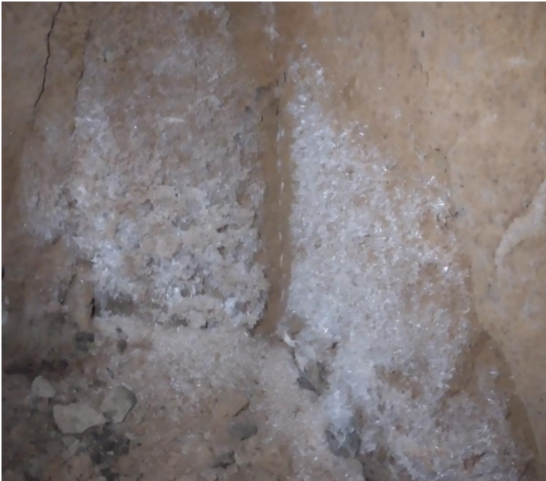
Image 1. Salt crystals are growing in an anthropogenic cave. Sample MIP1
