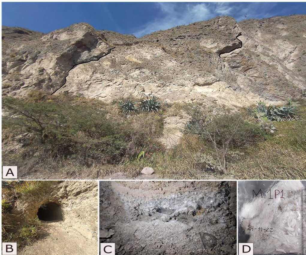
Figure 7. Outcrop with cracks near the Ambí River (See location in Figure 1) (A). Artificial channel (B). Crystallized salts in the ground (C). M1P1 Sample taken in the channel(D)
