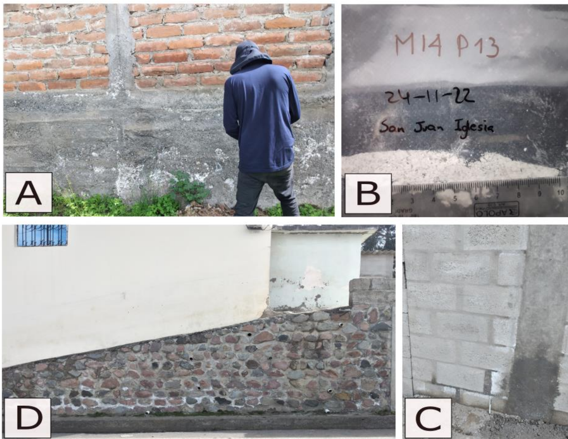
Figure 20. Taking crystals from a wall (A). The sample was taken M14P13 (B). White crystals are present at the base of a rock wall (C). Crystals are seen in a freshly built wall (D)
