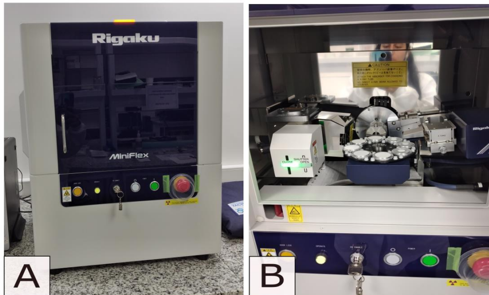
Figure 5. The X-ray diffraction (XRD) machine and the space within it.
