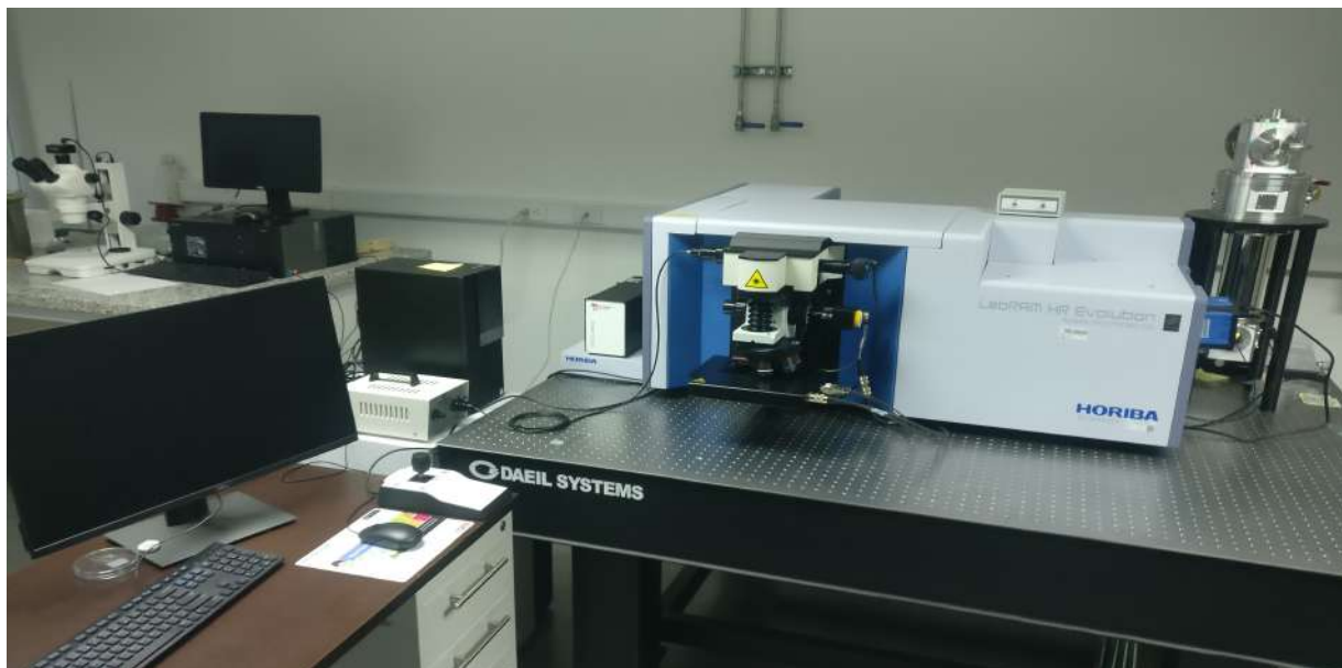
Figure 3.2: Horiba LabRam HR Evolution, Laboratory of characterization Yachay Tech University
