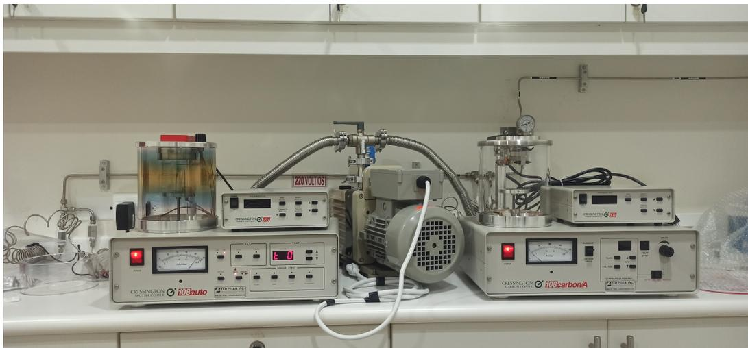
Figure 3.6: 108C Auto/SE Carbon Coater. Equipment used for sample coating prior to SEM characterization.
