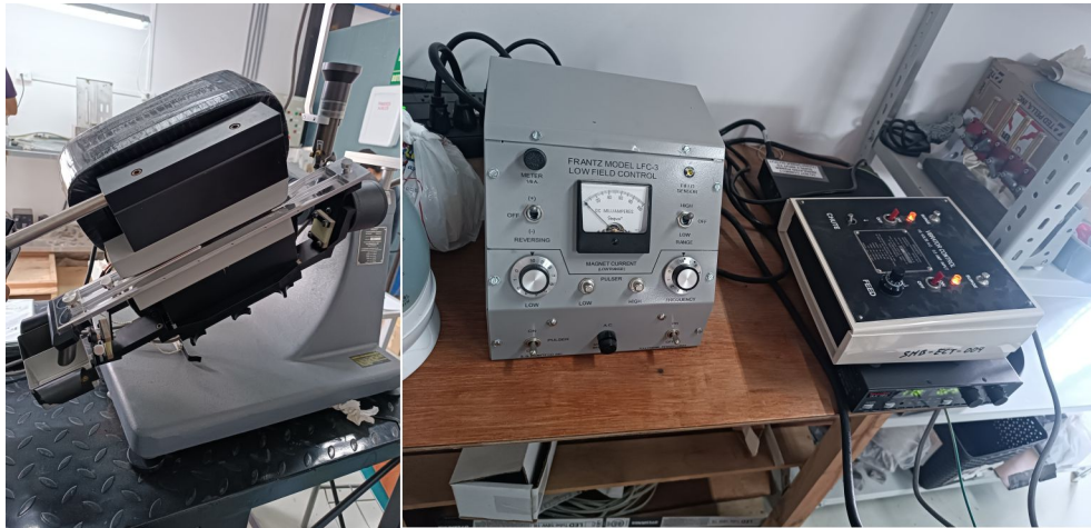
Figure 3.4: Magnetic separator Frantz model LB-1. It consists of a strong electromagnet that can produce controlled magnetic fields around a channel between two large magnets and a current and voltage regulator that allows us to control and monitor the magnetic field in which we separate our samples.
