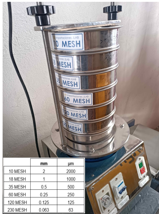
Figure 3.2: Sieving machine for the granulometric separation of the sands. Each level has its net size from 10 MESH to 230 MESH (the values in \mu\text{m} are reported in the attached table). The sand particles are separated by size using the vibration of the machine's base and passing through a series of fine nets.
