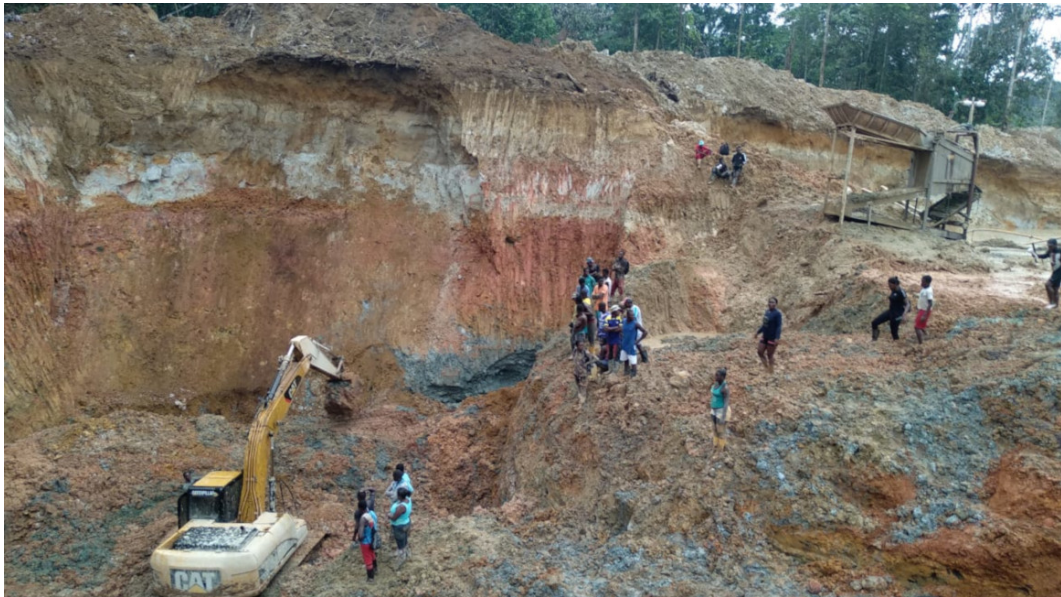
Figure 1.3: Photography published by Primicias EC ( primicias.ec ), an online journal of Ecuador. It shows how in San Lorenzo Canton, the illegal mining activity has grown, having big machinery and people working to extract the metal-rich material from the alluvial deposits on riverbanks.
