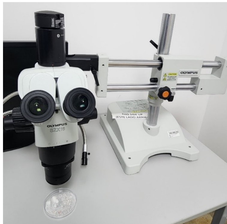
Figure 3.7: Stereomicroscope Olympus SZX equipped with an SC100 camera in which we captured the high-resolution imagery of the mineral grains.
