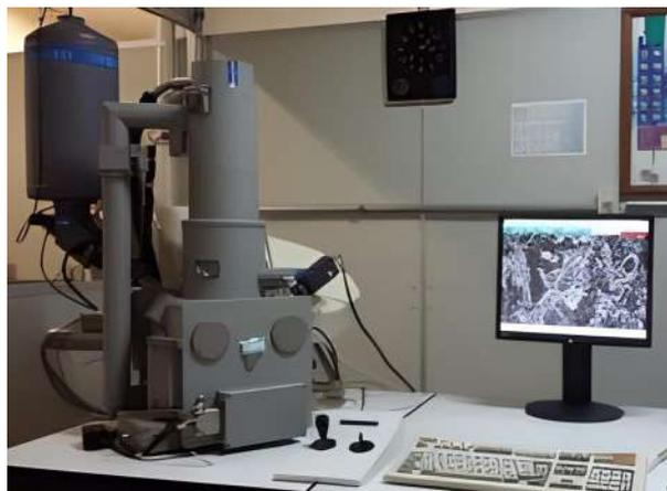
Figure 4.6: LEO model 440 Scanning Electron Microscope.
