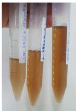
Figure 4.2: Sodium alginate crosslinking with genipin at concentrations of 0.25, 0.5, and 1 % (v/v) (left to right).
