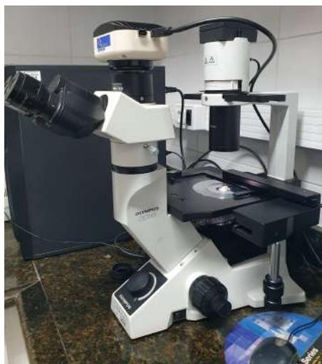
Figure 4.10: Olympus CKX41 Inverted Microscope.
