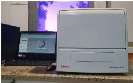
Figure 4.9: Thermo Scientific™ Varioskan™ LUX multimode microplate reader.
