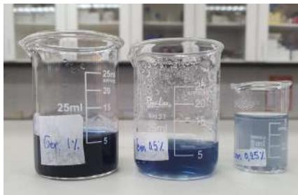
Figure 4.3: Hydrogels composites crosslinking with genipin at concentrations of 1, 0.5, and 0.25% (v/v) (left to right).
