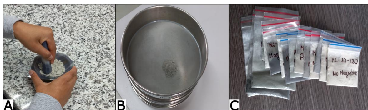
Figure 16. Sample pulverization. A) Pulverized hand. B) Sieved Samples. C) Ready samples.
