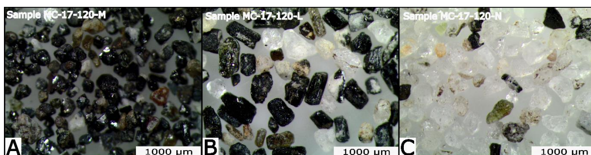
Figure 27. Images of result of magnetic separation of fraction collected of mesh 120 of sample MC-17. A) Magnetic fraction separates to magnitude of 0,35. B) Medium fraction separate to magnitude of 0,2. C) Non magnetic fraction separate to magnitude of 0,35.
