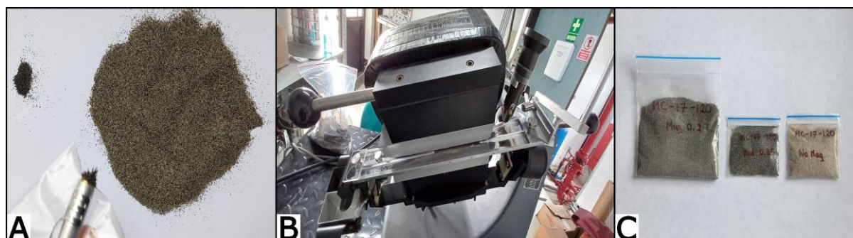
Figure 15. Magnetic separation. A) Manual separation used to neodymium magnetic. B) Frantz magnetic separator. C) Fractions separation.
