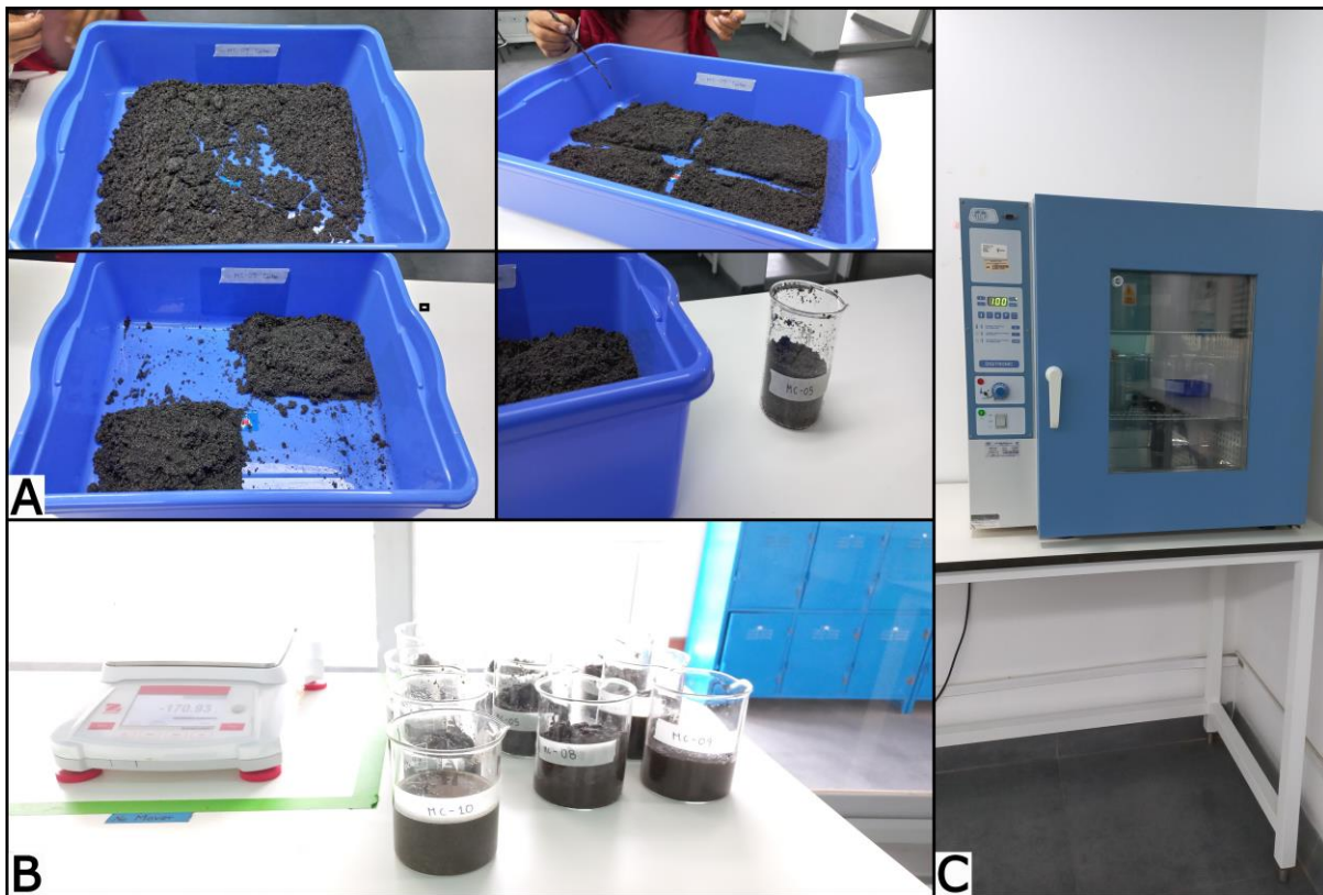
Figure 12. Process of sample drying. A) Applied to quartering method. B) Sample weighing. C) Laboratory stove
