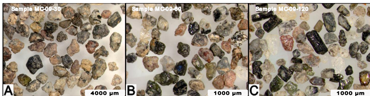
Figure 23. A) Fraction collected at 35 mesh with a high presence of lithic fragments and almost no minerals. B) Fraction collected at 60 mesh with high presence of lithic fragments and little presence of minerals. C) Fraction collected at 120 mesh with little presence of lithic fragments and high presence of minerals.
