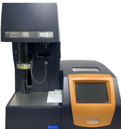
Figure 3.7: Thermogravimetric analyzer, TGA 55
