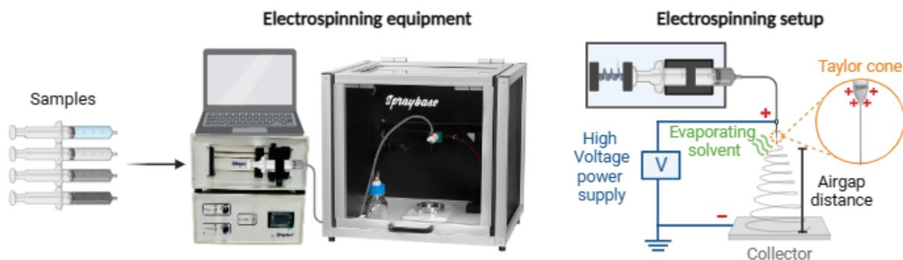
Figure 3.3: *SprayBase*<sup>TM</sup> electrospinning equipment and setup.
