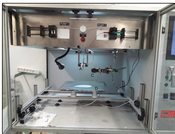
Figure 38. Electrospinning machines with principal components: needle, (b) pump, (c) camera and (d) square collector covered with aluminum.
