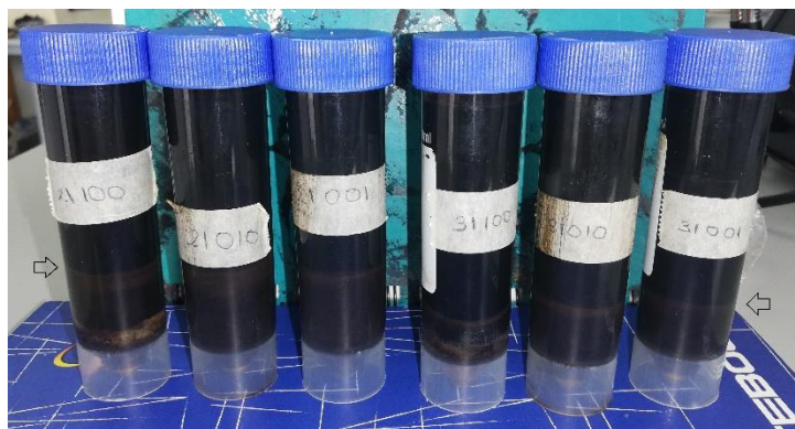
Fig26._ Emulsions 21YYY (left) and 31YYY (right) after centrifugations. Narrows indicate the upper level of emulsion layer.
