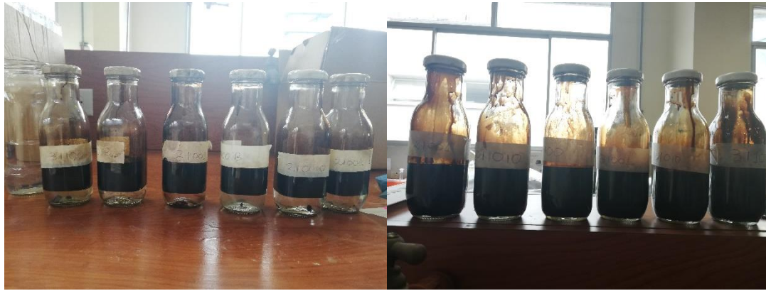
Fig 21._ Mixture of crude oil and formation water (left). Emulsions 31100, 31010, 31001, 21100, 21010, 21001 generated at 8000 rpm with a homogenizer (right). The first two numbers in the nomenclature refers to the volumetric ratio of crude oil and water and the other three to the volumetric percentage of formation water in the aqueous phase.
