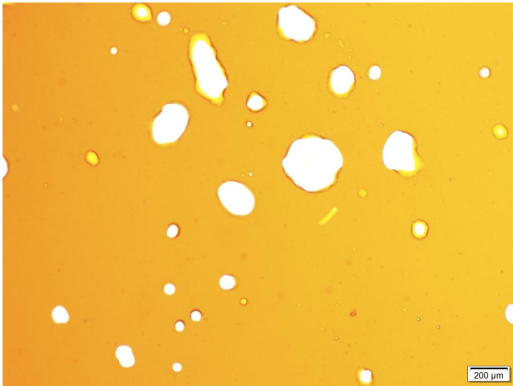
Fig 31._ Microphotography of emulsion 31001 (top), 31010 (medium) and 31100 (bottom) taken with a 4x zoom in the objective. Dispersed phase is water and the continuous phase is crude oil.
