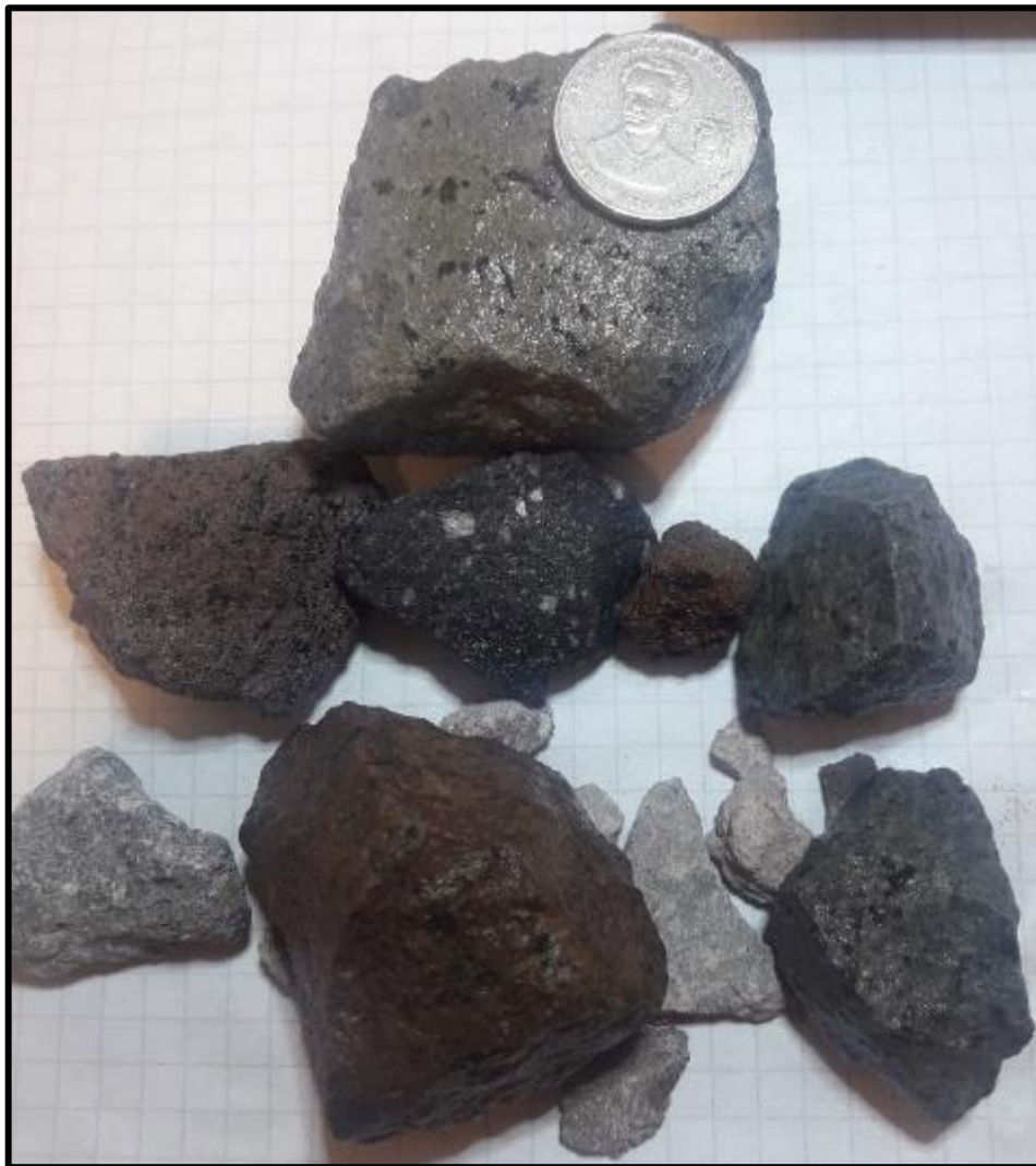
Figure 23. Ripio. Is known as Ripio at the mixture of rocks composed of: andesites, amphibole andesites, amphibole-pyroxene andesites, amphibole-plagioclase andesites and, tuffs, expended as aggregate by the concrete to produce concrete, employed in slabs and columns. To be considered as Ripio the size of rocks must be between 10 to 51 mm (Author).
