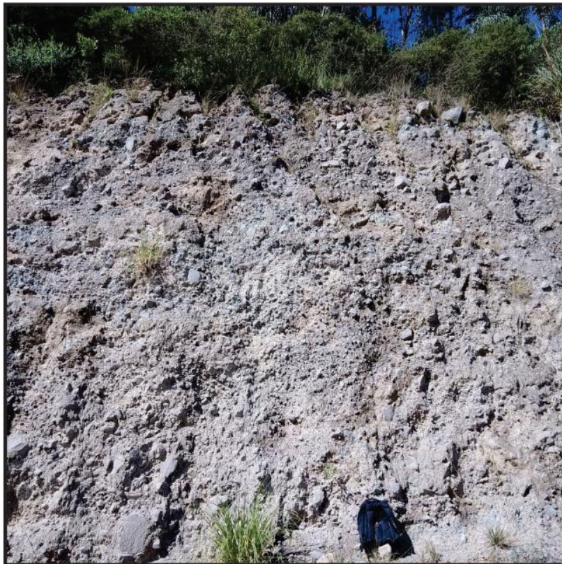
Figure 19. Block Facies Bf. The Bf shown in the figure belongs to a mined slope from the Cerro Negro quarry located in the east of the city. Here the Mf reaches up to 22 m. this consist of a matrix-supported massive deposit poorly sorted. The clast size varies from 3 to 45 cm (Author).
