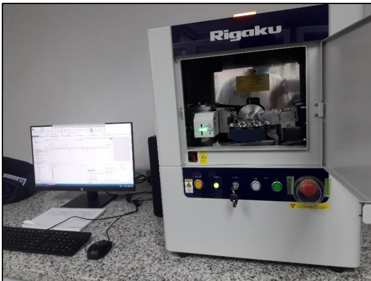
Figure 11. XR-D analyzer from the Yachay Tech university. The samples are scanning in the machine located at the right. Posteriorly, the data is digitalized and saved in the computer located to the left (Author).
