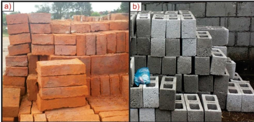
Figure 5. Terracotta and Concrete Bricks. a) shows the form of terracotta bricks employed to build the different infrastructure in Riobamba city. b) shows the form how concrete brick is exposed to be expended (Gavilanes & Santellan, 2016).
