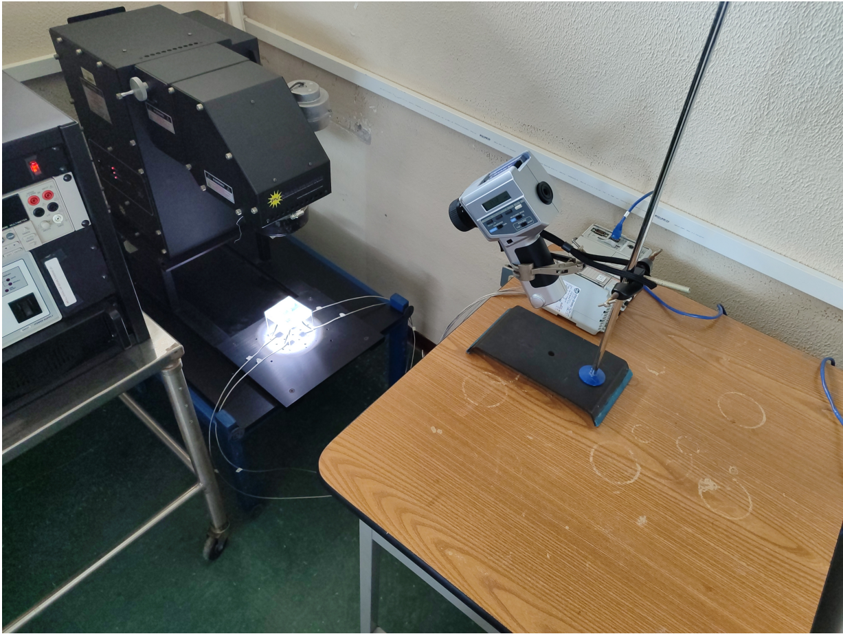
Figure 3.7: Solar chamber heat capture test of the samples and luminometer setup.
