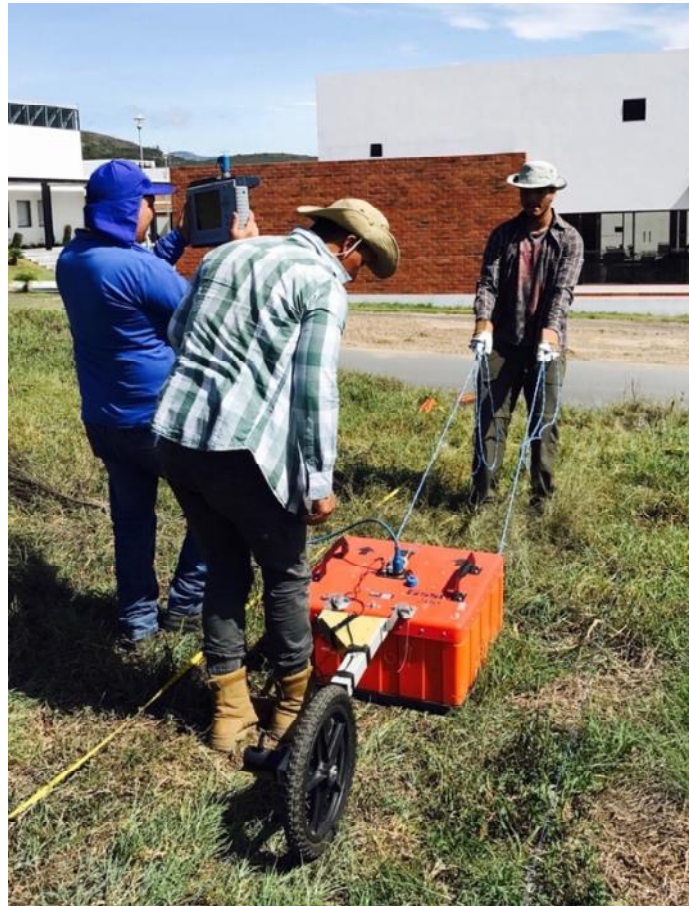
Figure 4. GPR equipment of EPMAPS in the field. Diego Guanotuña is holding the control unit in his hands on the left of the photo. The main sending/receiving antenna is in the orange box being pulled by Gustavo Béjar (right). The box is connected to a survey wheel which simultaneously measures the distance.
