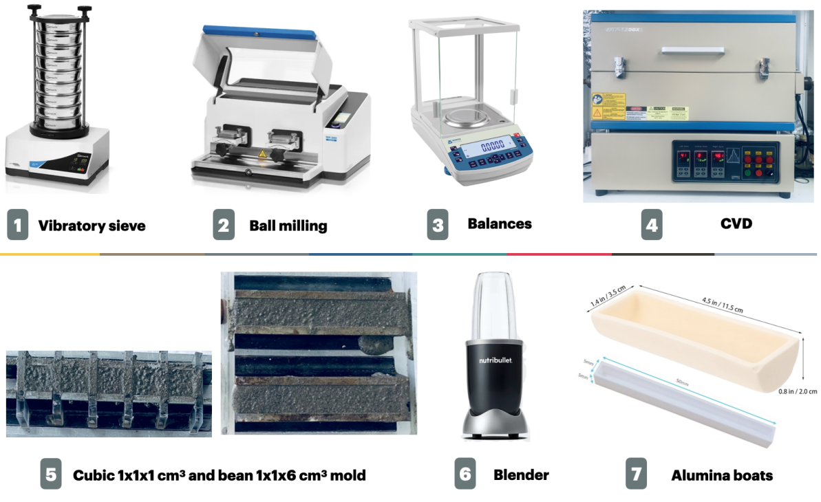
Figure 4.1: Main equipment's used for the synthesis of nano-engineered cement and for specimen preparation
