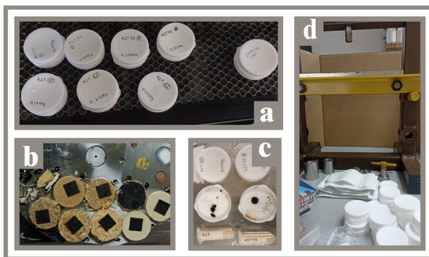
Figure 5.2: Images of samples before, during, and after the synthesis process. a. Samples before the laser ablation process, image taken in the laser cutter cabin. b. XPS sample holder with the samples prepared before the measurements. c. Image of synthesized samples A1T and A1T75 after the surface scraping. d. Mechanical press stage where pills were prepared, and samples on its containers.,
