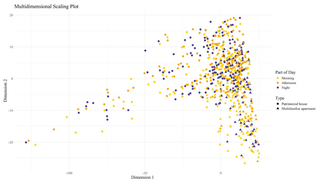
Figure 5.3: Multidimensional scaling plot, showing the relationships between radon, temperature, and relative humidity. Patrimonial houses in circle, Multifamiliares apartments in triangle. Colors represent the part of the day in which the measurements were taken, in yellow for morning, in orange for afternoon, and in purple for night.
