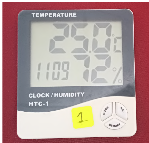
Figure 4.9: HTC-1 thermometer and hygrometer device. Photo taken by author.
