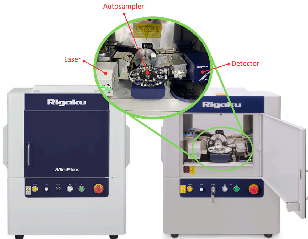
Figure 3.9: Mini Flex (G6) X-ray Diffraction. Diffractometer used for identifying the phase of SiC grains.
