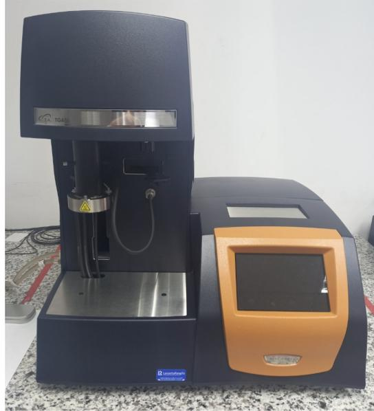
Figure 3.7: Thermogravimetric Analyzer.
