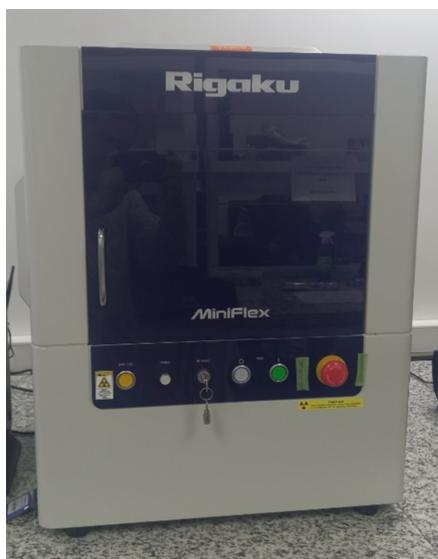
Figure 3.6: X-ray Diffractometer.
