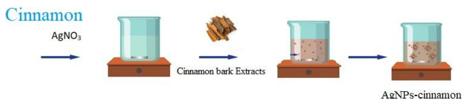
Figure 10 Scheme of synthesis of silver nanoparticles using cinnamon bark extract
