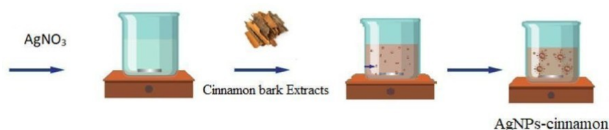
Figure 3. Scheme of synthesis of silver nanoparticle from cinnamon bark extract.
