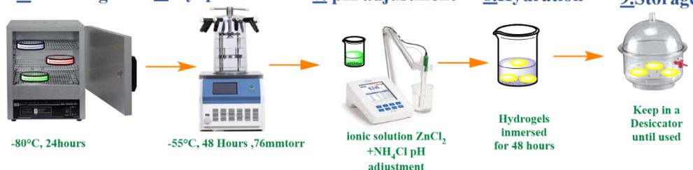
Figure 3. Synthesis of chitosan-starch hydrogels using physical crosslinking techniques.
