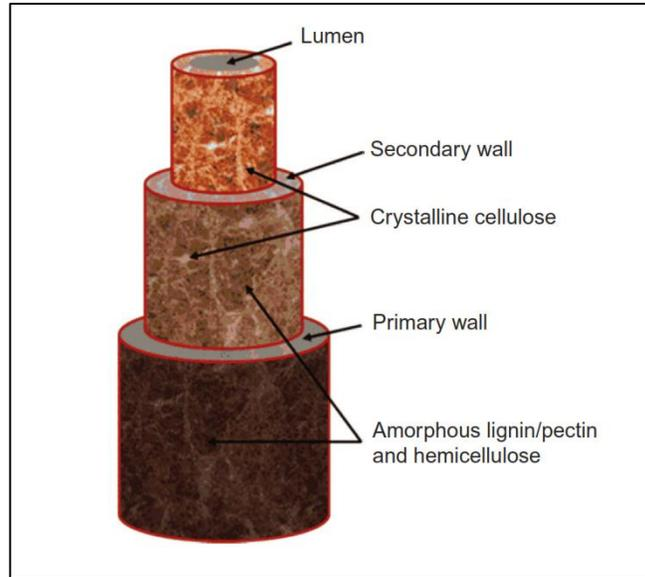
Figure 1.3 Structure of a plant fiber. Image extracted from: Thomas S, Paul S, Pothan L, Deepa B. *Natural Fibres: Structure, Properties and Applications. Cellulose Fibers: Bio- and Nano-Polymer Composites.* 2011:3-42.
