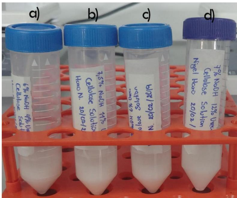
Figure 3.2 CC cellulose solution at a concentration of 4.16 wt% in low concentrations of precooled at 0 °C NaOH/urea aqueous solution. (a) CC cellulose solution at 6/4 wt% solvent concentration, (b) CC cellulose solution at 7.5/11 wt% solvent concentration, (c) CC cellulose solution at 5/6 wt% solvent concentration and (d) CC cellulose solution at 7/12 wt% solvent concentration
