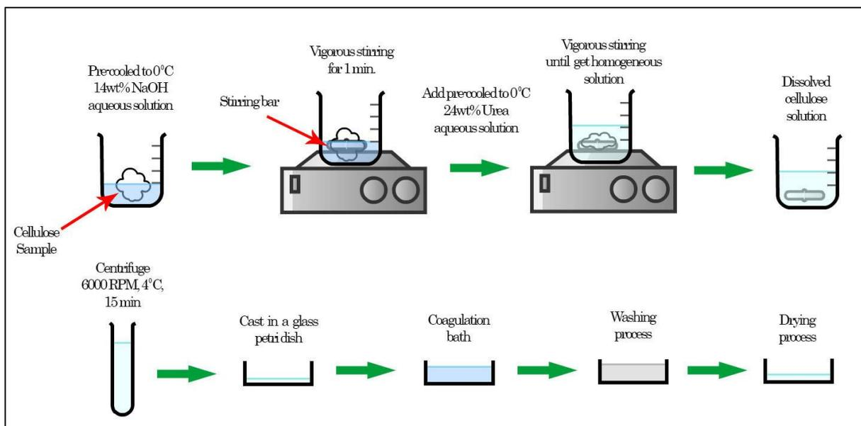
Figure 2.1 Two- step scheme for preparation of regenerated cellulose films from 14wt% NaOH / 24wt% Urea aqueous solution.
