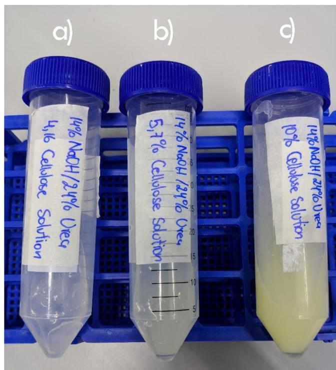
Figure 3.5 Influence of the cellulose concentration on the transparency of the CC cellulose solution from 14/24 wt% NaOH/urea aqueous solution. (a) cellulose solution at a concentration of 4.16 wt%; (b) cellulose solution at a concentration of 5.7 wt%; and (c) cellulose solution at a concentration of 10 wt%.
