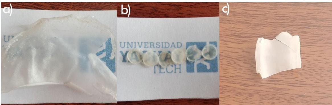
Figure 3.8 RC films obtained from 14/24 wt% NaOH/urea aqueous solution at different CC cellulose concentrations, regenerated with 80 v% ethanol. (a) Film obtained from a cellulose concentration of 4.16 wt%, (b) film obtained from a cellulose concentration of 5.7 wt%, (c) film obtained from a cellulose concentration of 10 wt%.
