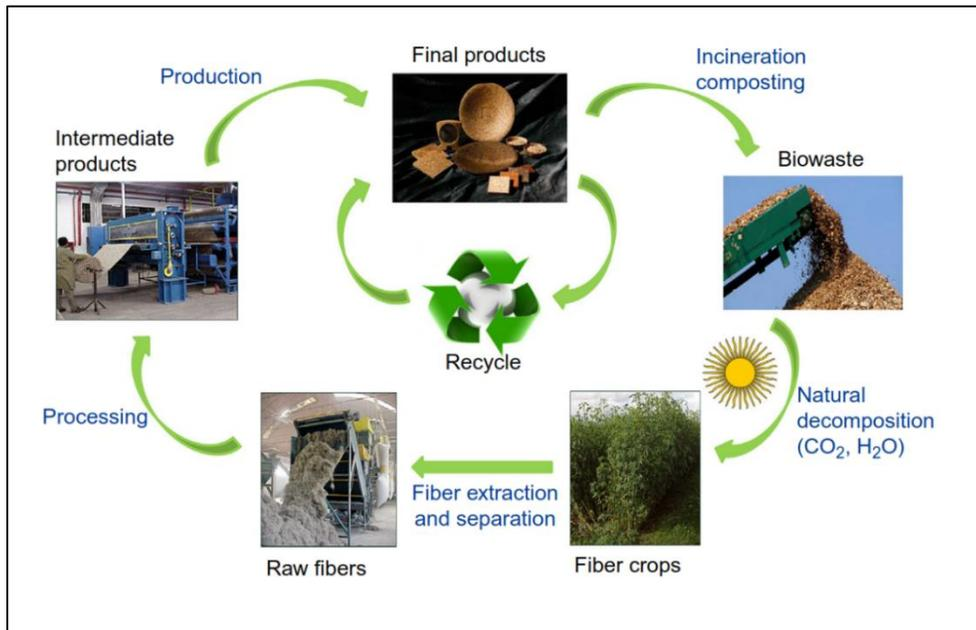
Figure 1.2 Life cycle of natural fibers. Image extracted from: Bhattacharyya D, Subasinghe A, Kim N. *Natural fibers: Their composites and flammability characterizations*. 2019.
