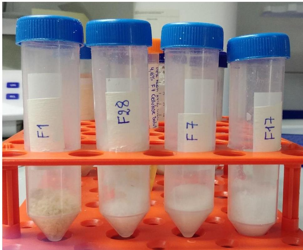
*Figure 3.1 Cellulose fibers extracted from natural sources, after the purification and drying process. from left to right, cellulose fibers F1, F28, F7 and F17.*
