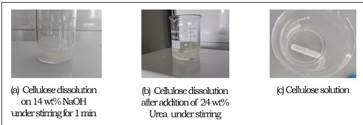
Figure A.2 Dissolution of cellulose through the two-step method under 14/24wt% solvent concentration., cellulose is dissolved first in NaOH 14 wt% aqueous solution pre-cooled to 0 °C with stirring for 1 min then urea 24 wt% aqueous solution pre-cooled to 0 °C is added immediately to the mixture under vigorous stirring until a homogeneous solution is achieved.
