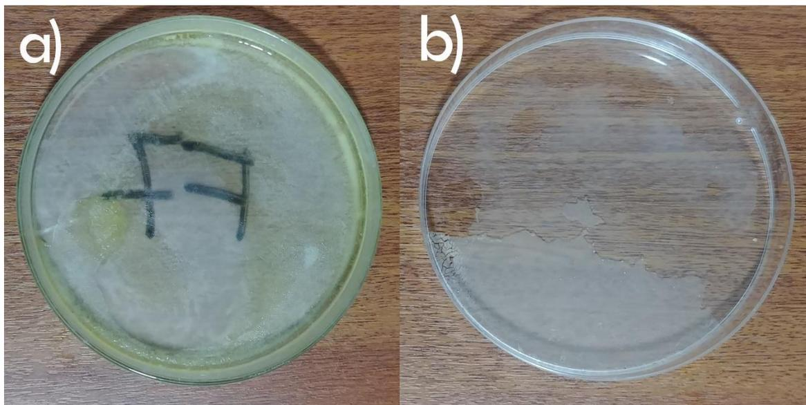
Figure 3.10 Regeneration of cellulose fiber films from 4.16 wt% cellulose solutions, 14/24 wt% NaOH/urea aqueous solution and 80 v% ethanol bath. (a) Remains of F7 film after having extracted the excess ethanol from the coagulation bath, (b) F28 film obtained after washing process and drying process at room temperature.
