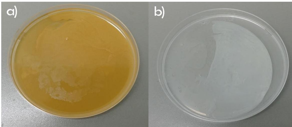
*Figure 3.12 Regeneration of "recoverable" films of a 5.7 wt% cellulose fiber solution from 14/24 wt% NaOH/urea aqueous solution and 80% ethanol coagulation bath. (a) C1 film after 20 min of coagulation, (b) C2 film after 20 min of coagulation.*
