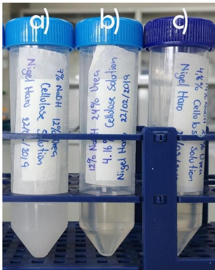
Figure 3.3 CC cellulose solution at 4.16 wt% cellulose concentration in high concentrations of NaOH/urea aqueous solution precooled at 0 °C. (a) CC cellulose solution at 7/12 wt% solvent concentration, (b) CC cellulose solution at 12/24 wt% solvent concentration and (c) CC cellulose solution at 14/24 wt% solvent concentration.
