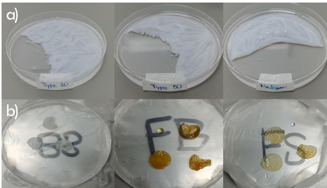
Figure 3.13 RC films usable from a cellulose concentration of 5.7wt%, 14/24wt% NaOH/urea aqueous solution and coagulation with ethanol at 80 v%. (a) From left to right: T20, T50, TM usable films obtained from industrial type cellulose, (b) From left to right: BS, FB, FS usable films obtained from natural cellulose fibers.
