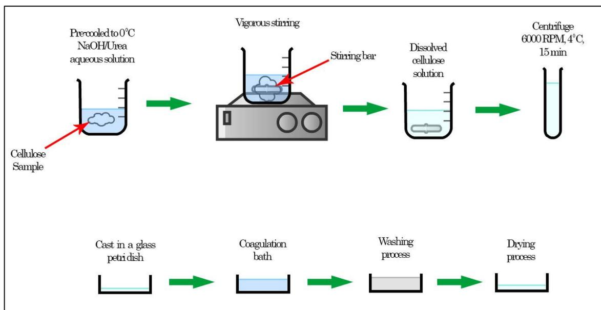
Figure 2.2 One step scheme for preparation of regenerated cellulose films from NaOH/urea aqueous solution.
