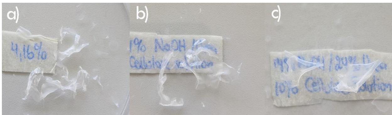
Figure 3.7 RC films obtained from 4.16wt% CC cellulose solutions, coagulation bath with 100 v% isopropanol and 14/24 wt% NaOH/urea aqueous solution (a) transparent CC film after 1 h of drying, (b) Shrinkage of CC film after 3 days at room temperature.
