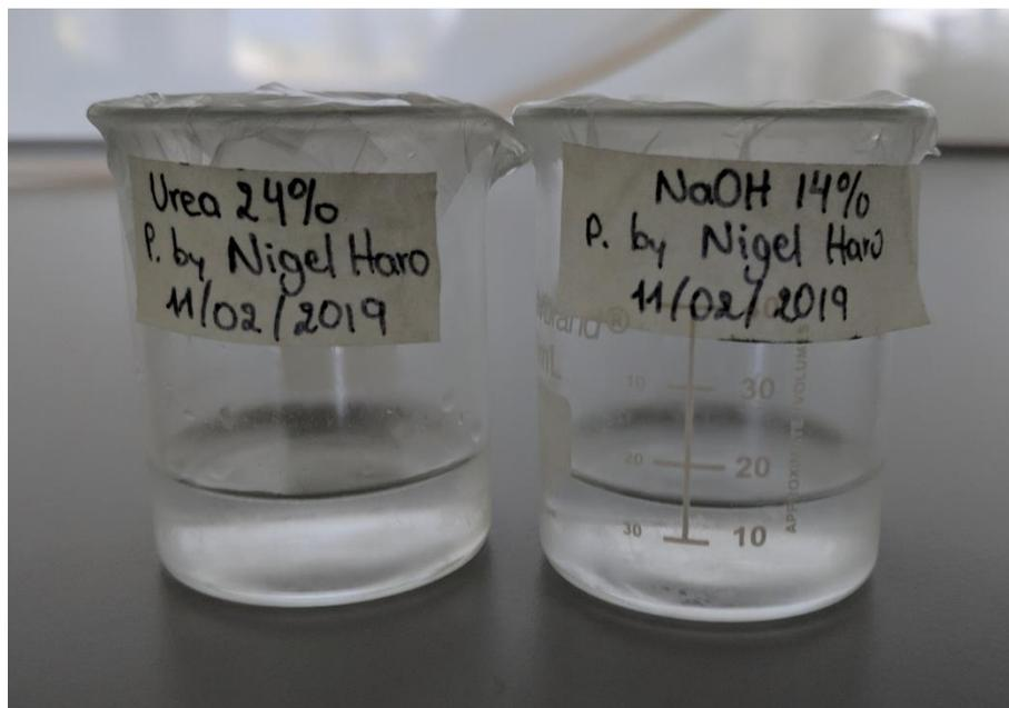
Figure A.1 Low temperature aqueous solutions. (a) 24wt% urea precooled at 0 °C, (b) 14wt% NaOH precooled at 0 °C
