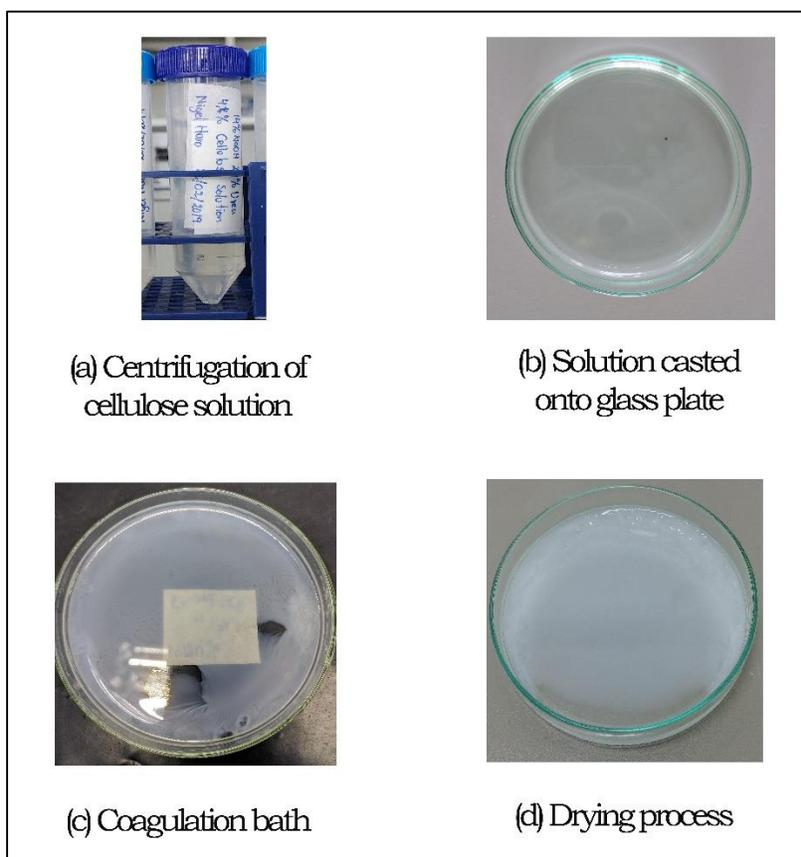
Figure A.3 Process for the regeneration of the film. (a) Centrifugation of the cellulose solution for degassing, (b) the solution is spread on a glass petri dish, (c) the solution is subjected to a coagulation bath for regeneration, (d) the regenerated film is washed with distilled water and let to dry at room temperature.
