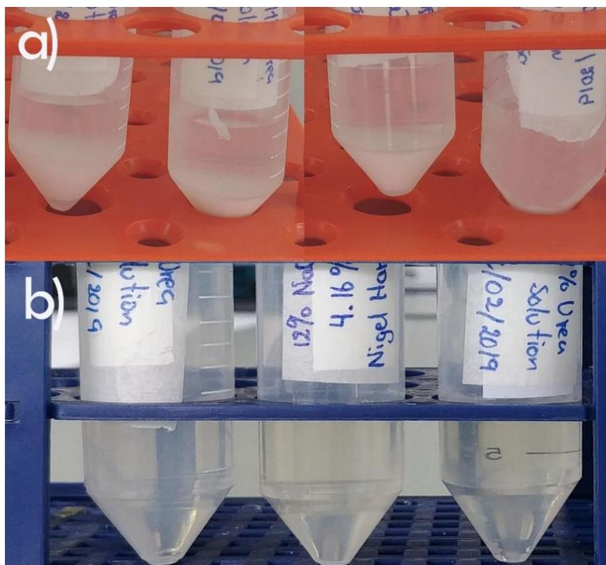
Figure 3.4 CC dissolved cellulose solutions at different cellulose solutions after centrifugation at 6000 rpm at 4 °C for 15 min. (a) From left to right: CC cellulose solutions from 6/4 wt%, 7.5/12 wt%, 5/6 wt% and 7/12 wt% NaOH/urea low concentration aqueous solution. (b) From left to right: CC cellulose solutions from 7/12 wt%, 12/24 wt% and 14/24wt% NaOH/urea low concentration aqueous solution.
