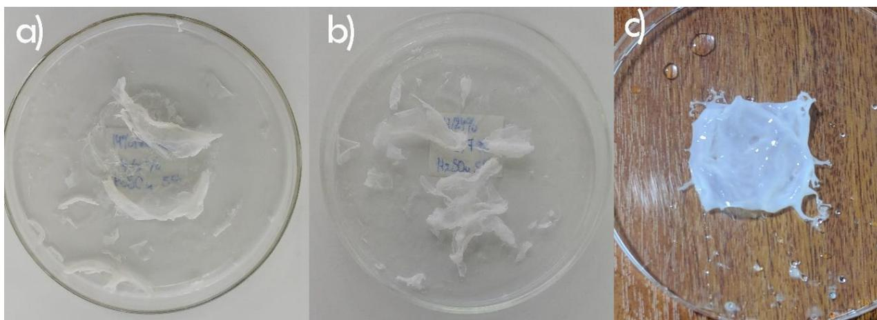
Figure 3.6 RC films obtained from coagulation with 5 v% sulfuric acid of CC cellulose solutions, 14/24 wt% NaOH/urea aqueous solution and different CC cellulose concentrations. (a) RC film obtained from 4.16 wt% cellulose solution, (b) RC film obtained from 5.7 wt% cellulose solution, (c) RC film obtained from 10 wt% cellulose solution.
