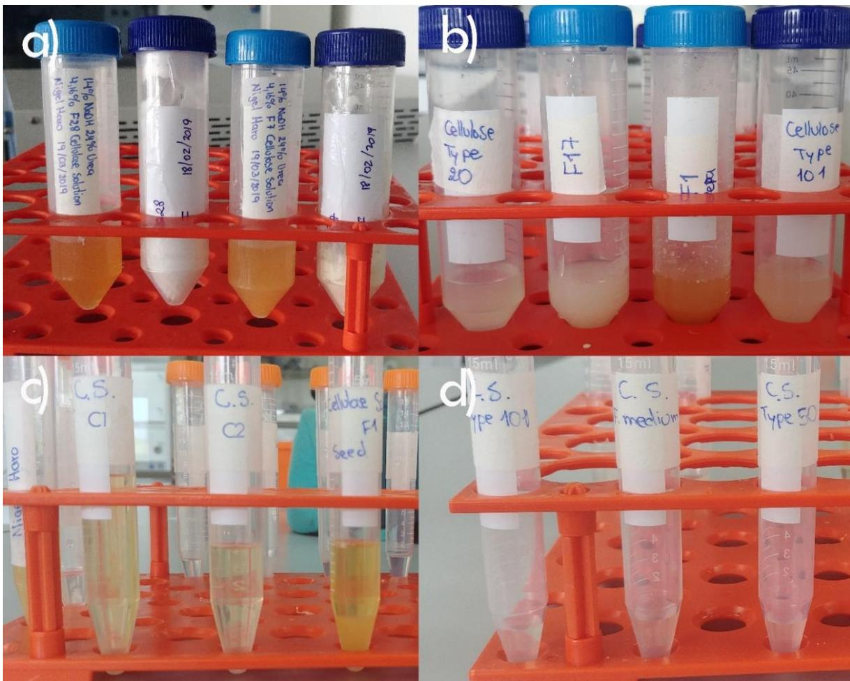
Figure 3.9 Cellulose dissolution of different sources from 14 wt% NaOH/24 wt% urea aqueous solution. (a) Cellulose fibers F28 and F7 solutions with their corresponding white cellulose fibers, (b) cellulose solution of cellulose fibers F17, F1 and industrial type cellulose T20, T101, (c) dissolution of cellulose fibers after centrifugation at 6000 rpm at 4 °C for 15 min, (d) industrial type cellulose solutions after centrifugation at 6000 rpm at 4 °C for 15 min.
