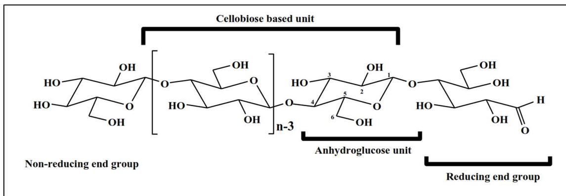
Figure 1.5 D-anhydroglucopyranose units (AGU), connected by  $\beta$  (1-4)-glycosidic bonds. Image extracted from [14]
