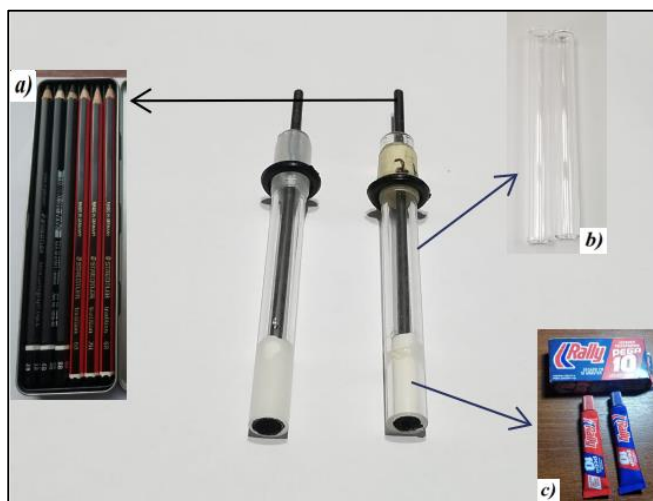
Figure 7. Construction of 2H-graphite electrode. a) Commercial 2H-pencil graphite (Staedtler, Germany), b) Glass tubing, and c) Epoxy resin.
