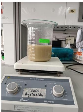
*Figure 15. Pillarization of CZY-305 clay*
