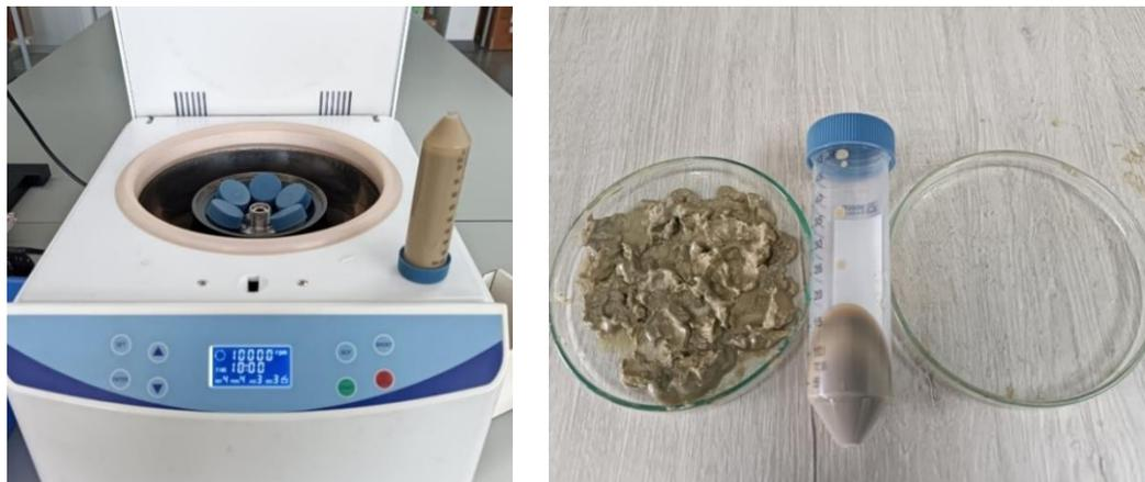
**Figure 12.** Centrifugation of preprocessed clays.
