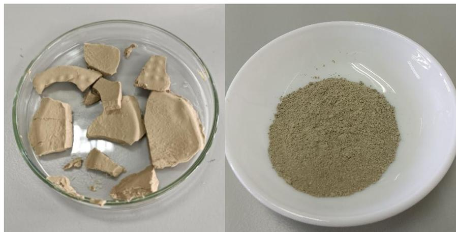
*Figure 18. Drying and calcining*
