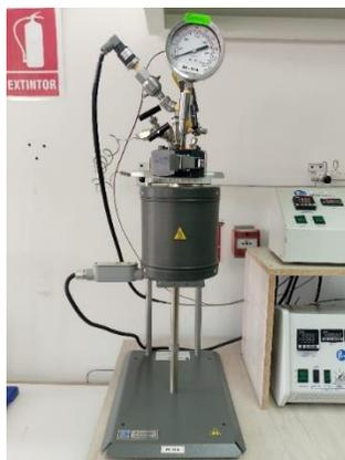
***Figure 27. Non-stirred reactor***
