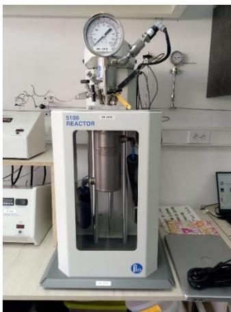
*Figure 26. Jacket stirred reactor*
