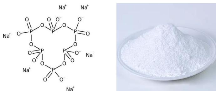
**Figure 8.** Powder and structure of sodium hexametaphosphate [ $\text{Na}_6(\text{PO}_3)_6$ ] (SHMP).
