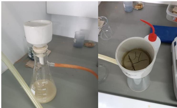
*Figure 17. Washing and filtering of pillared CZY-305 clay*
