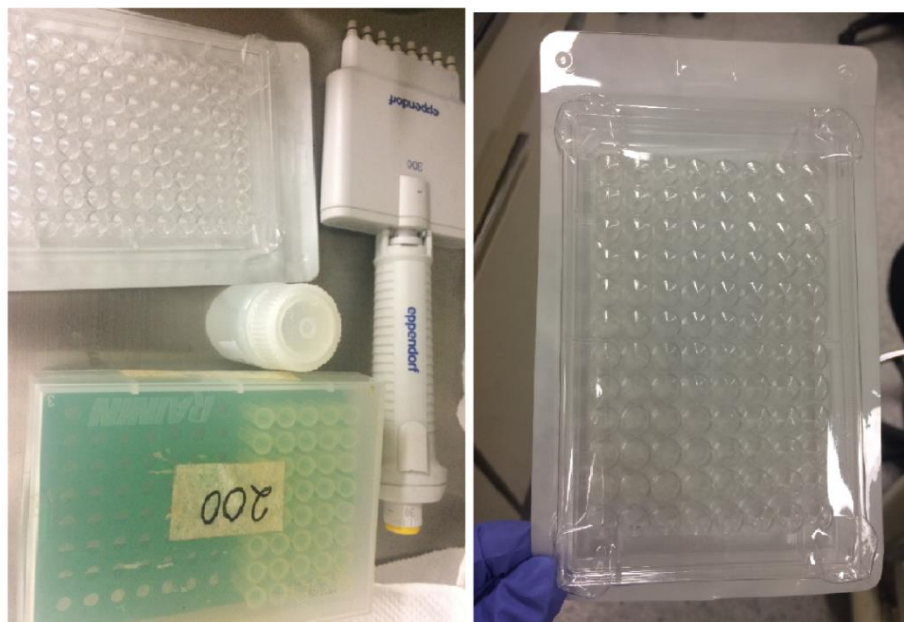
Figure 18. Elisa Plate, Micropipette of eight points of 100 \mu l and tips (Materials for sample preparation)
