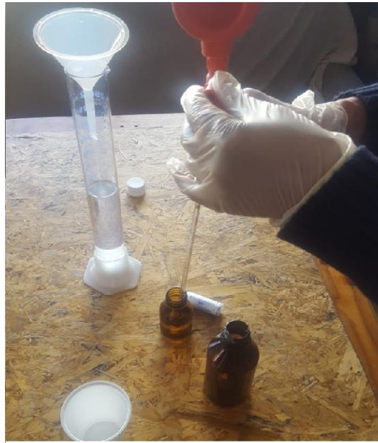
Figure 15. Experimental assembly to collect rain water sample.
