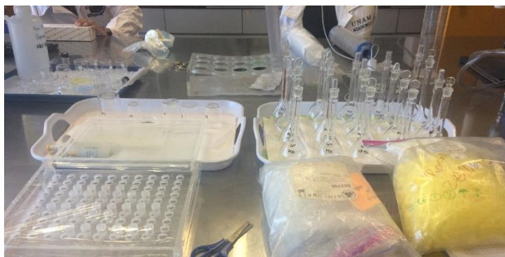
Figure 23. Sample preparation for Atomic absorption analysis.
