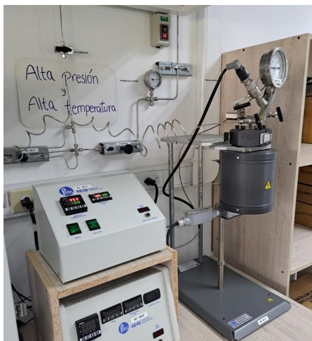
Figure 13. CO 2 capture reactor doing the absorption process with the clay sample.
