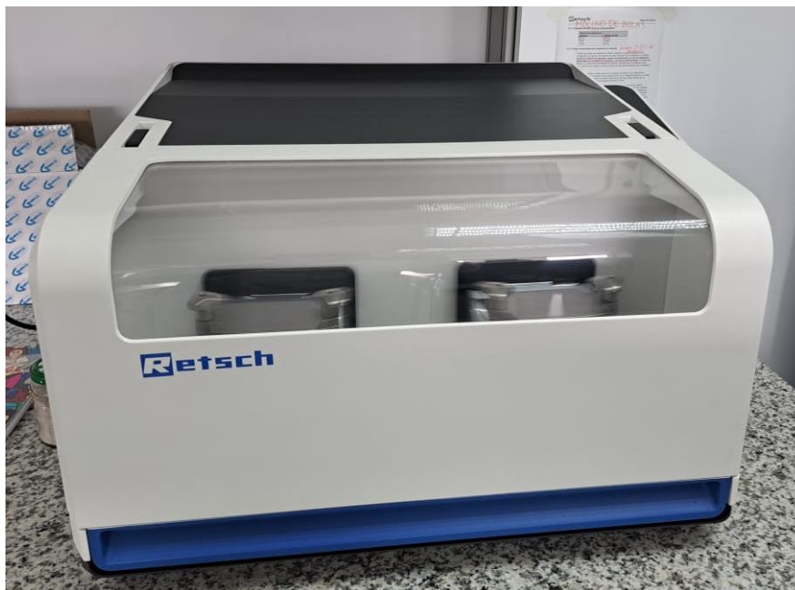
Figure 7. Retsch milling ball equipment reducing the sample particle size.
