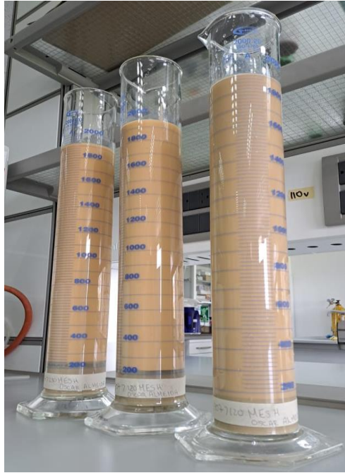
Figure 14. Clay sedimentation and layer separation in 2 L graduated cylinder for 21 days.
