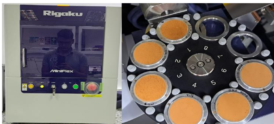
Figure 10. X-ray diffractometry and goniometer with 6 samples.
