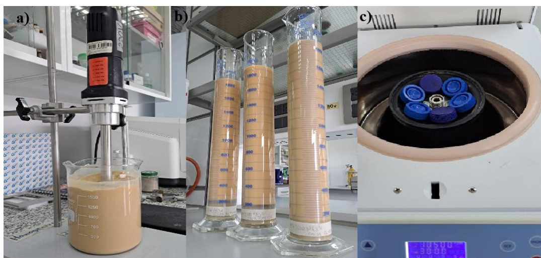
Figure 6. Purification process of clays COL-307 and CZP-303. a) Homogenization. b) Layer segregation. c) centrifugation of less dense layer.
