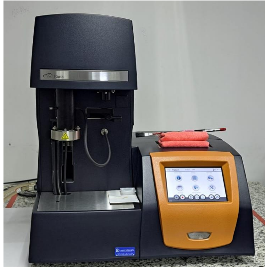
Figure 11. TGA equipment with a zinc oxide sample after CO 2 adsorption.
