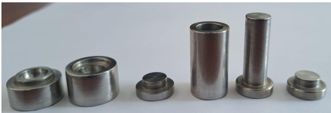
Figure 8. Spherical and cylindrical molds with their respective parts.
