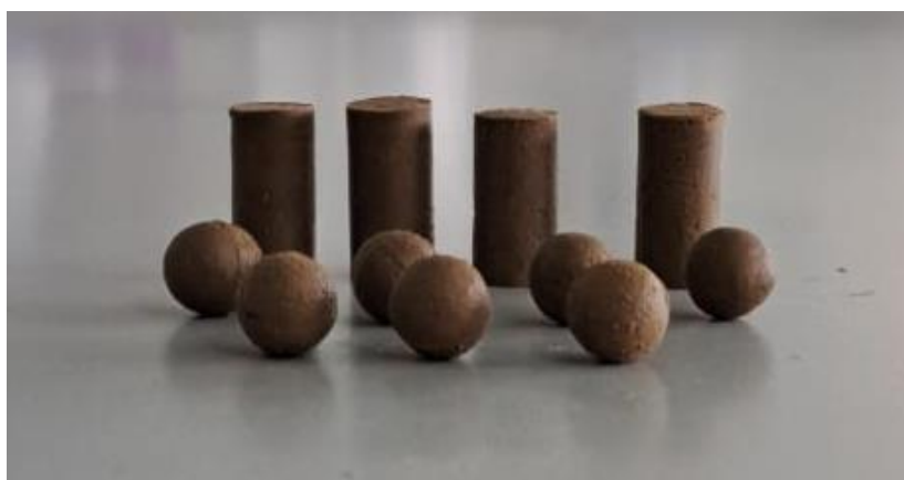
Figure 9. Spherical and cylindrical pellets of COL-307 after unmolding.
