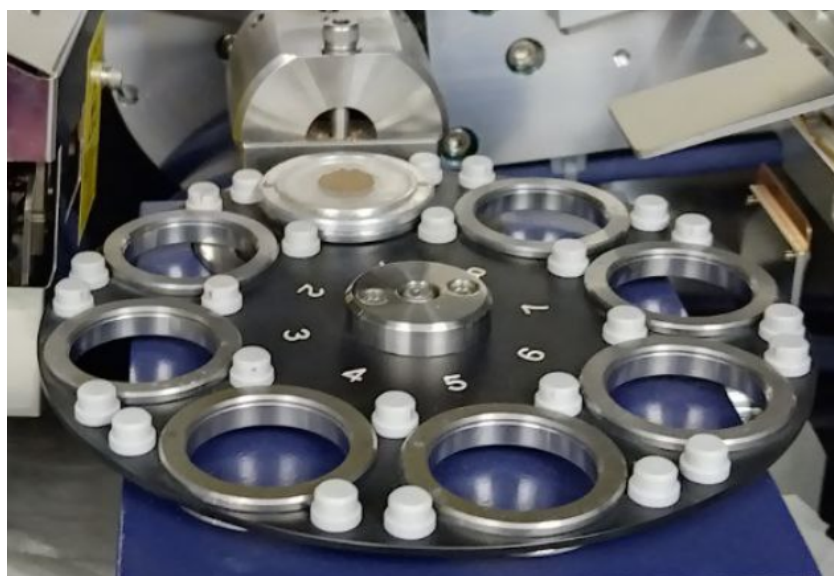
Figure 3.4: Rigaku MiniFlex 600 X-ray Diffractometer taking the measure of the first synthesis sample
