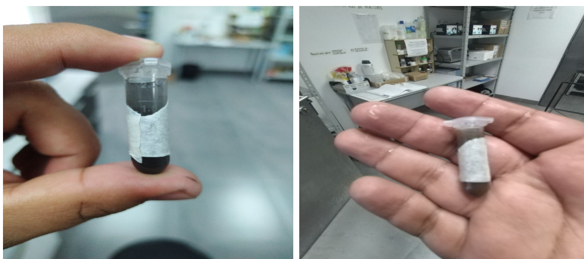
(a) 350 °C calcinated sample diluted in chitosan before to ultrasound treatment. (b) 350 °C calcinated sample diluted in chitosan after to ultrasound treatment.
