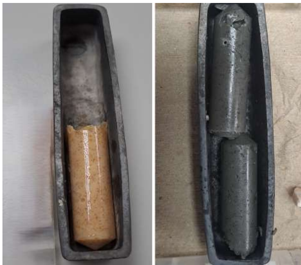
Figure 4.7: Image of oSiC (left) and oSiCZC (right) before calcination.
